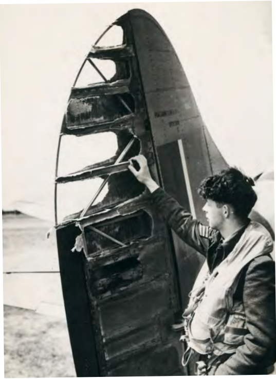
Above Sgt Bob Cole of 3 Squadron surveys the burned tail of his Tempest after flying through an exploding V-1. KEY COLLECTION
