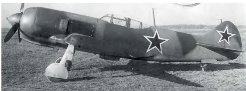
Above Lavochkin La-5FN 'White 72' featured an upgraded M-82FN powerplant developing almost 1,850hp. The type's distinctive strake on top of the engine cowling is evident.
