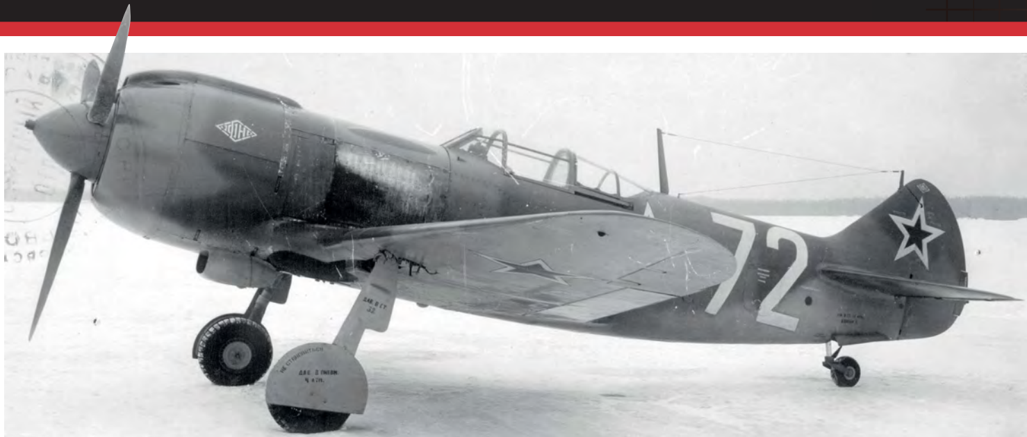
Above Lavochkin La-5FN 'White 72' featured an upgraded M-82FN powerplant developing almost 1,850hp. The type's distinctive strake on top of the engine cowling is evident.
