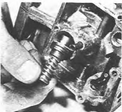
10.5a Note the compressible washer
