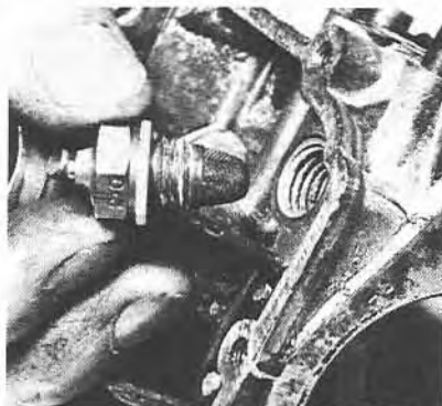
10.4 Use a new aluminium washer for the needle valve
