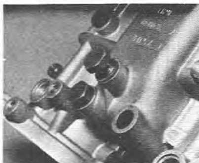
6.13 Removing the drain plugs (triple choke type)
