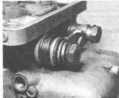
5.41 Removing the secondary shaft retaining nut
