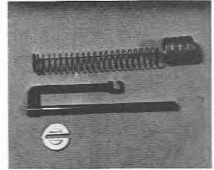
5.17 Accelerator pump components (twin choke type)
