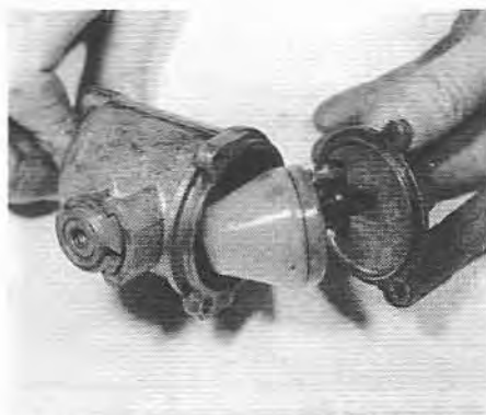
7.16 Removing the float chamber lid
