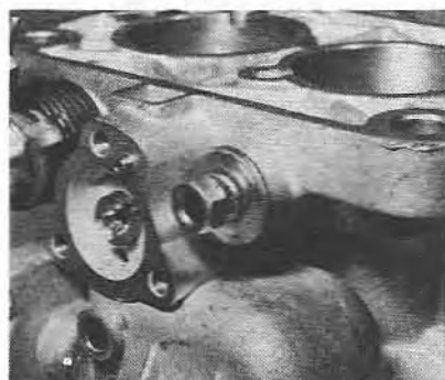
5.51 Removing the secondary throttle shaft nut
