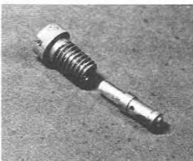
6.15b An idling jet and holder (triple choke type)
