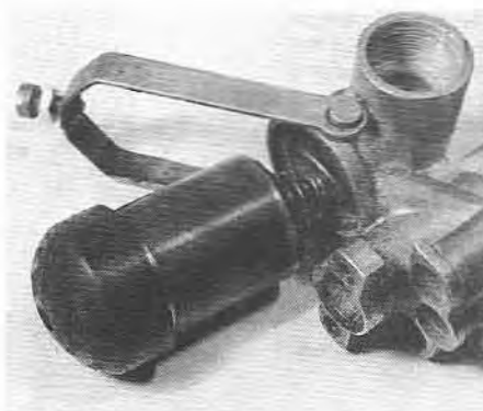
5.6A Removing the solenoid
