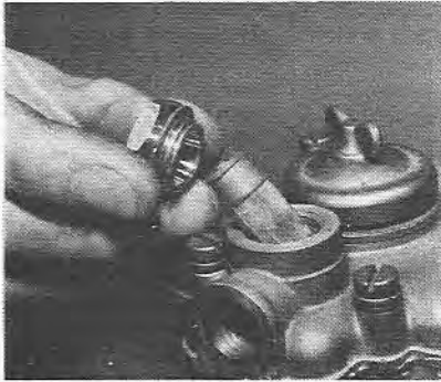
5.2 Removing the fuel filter
