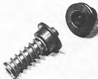
10.5 The upper jet assembly before insertion
