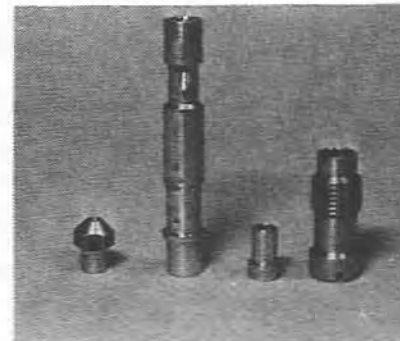
5.15 Component parts of the emulsion tube assembly
