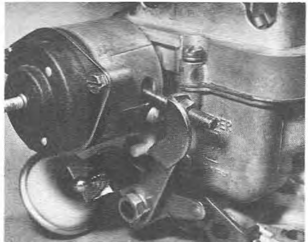
8.11 Showing the throttle lever and the fast idle adjusting screw
