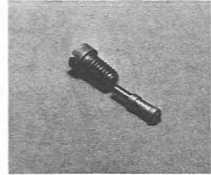
5.11b Idling jet and holder (DFAV type)
