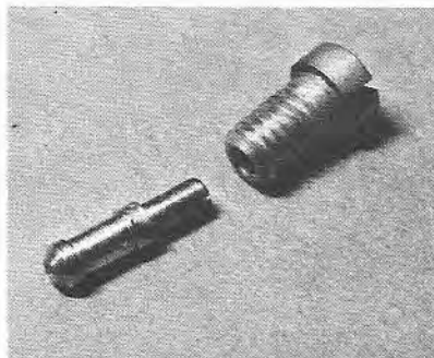
5.18 An idling jet separated from its holder
