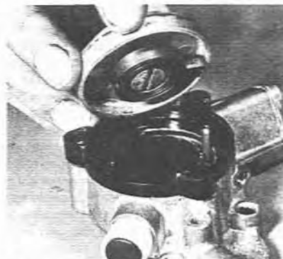
4.4 Fitting: Note the spring position
