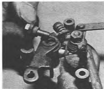
6.30 Removing the fast idle lever (DGAS type)
