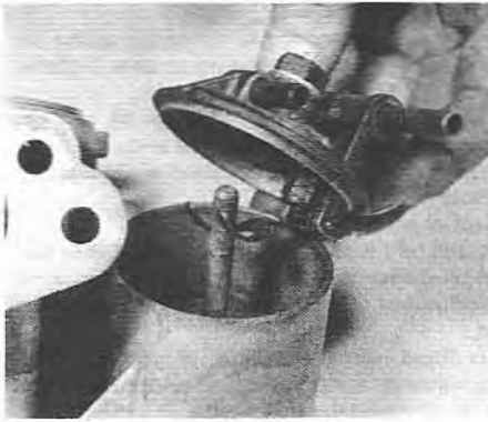
6.13 Removing the hose connection type float chamber lid
