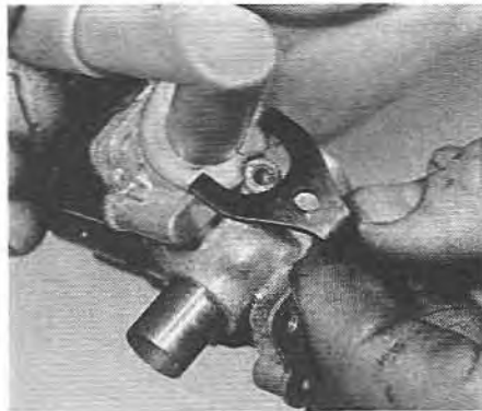
11.19A Air inlet stub and clamp removal
