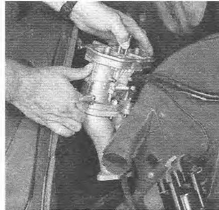
5.23 Install the left side carburetor first
