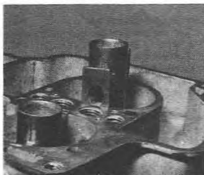
5.32a Removing an auxiliary venturi
