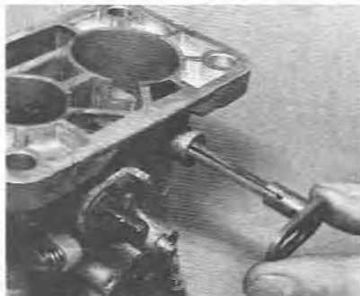
5.42 Withdrawing the secondary shaft from the carburettor body
