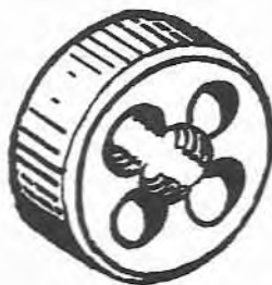
Fig. 4.4 Typical thread die
