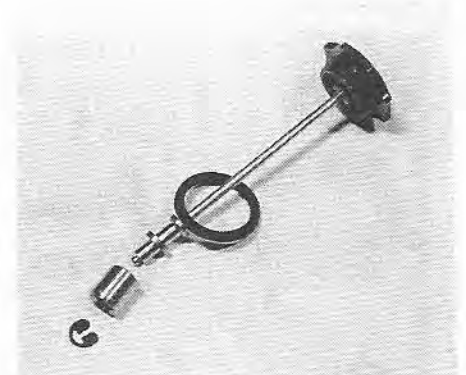
9.4B Dismantled damper rod valve
