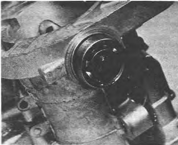
7.9 Fitting the throttle spindle bearing
