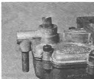
5.2b Removing the fuel filter
