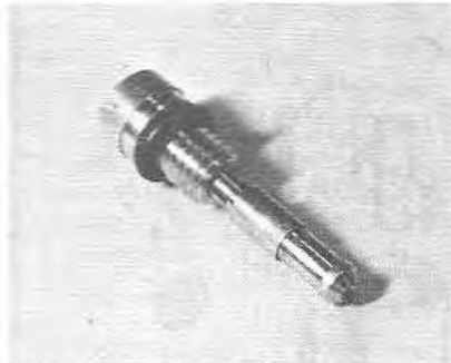
5.16b Separating an idling jet from its holder
