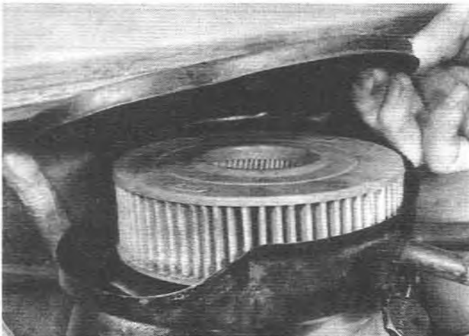
Fig. 3.4 Checking the air filter element in a SU carburetor
