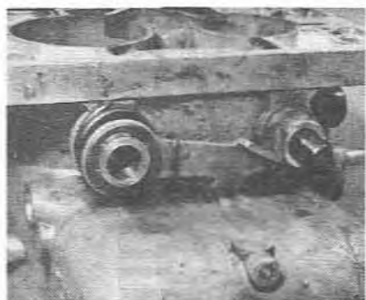
7.5 Correct assembled position of the accelerator pump control lever
