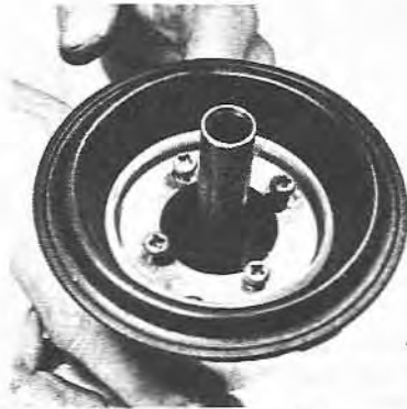
10.12b Tighten the four screws progressively
