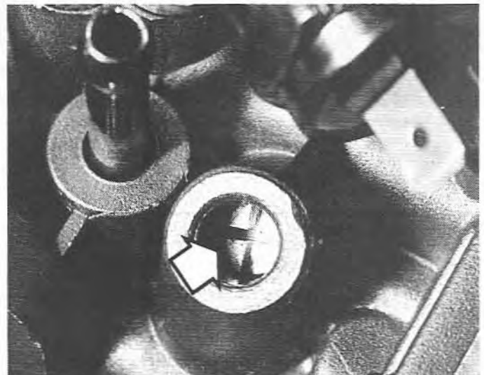
14.8A Mixture adjusting screw location (arrowed)
