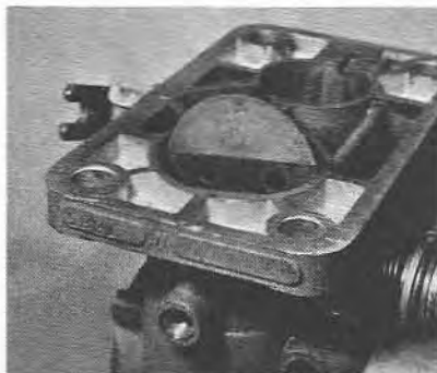
5.36 Removing the secondary throttle valve
