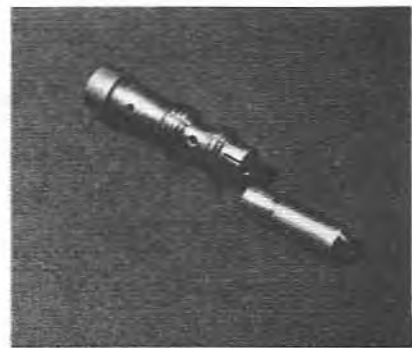
5.14b The idling jet and holder (twin choke type)
