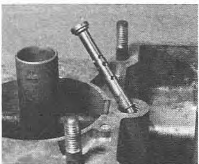
6.16b Removing an emulsion tube (triple choke type)
