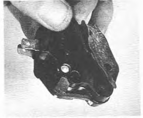
13.6D Removing the gasket from the delay valve
