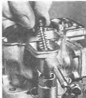
5.27b Removing the vent solenoid valve (USA types)
