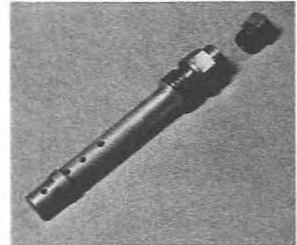
5.16 Location of an air corrector jet in an emulsion tube
