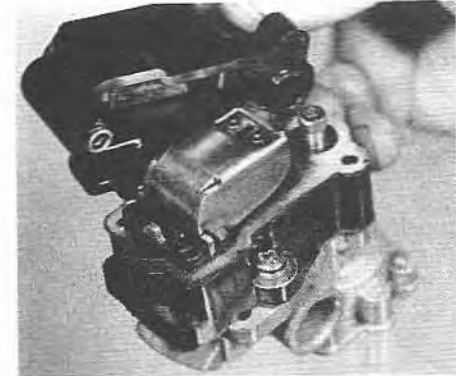
11.20 Valve body cover removal
