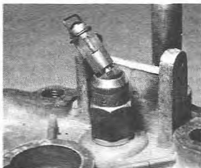
5.7 Removing the needle from the needle valve
