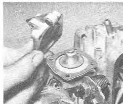
5.24a Removing the accelerator pump cover ...
