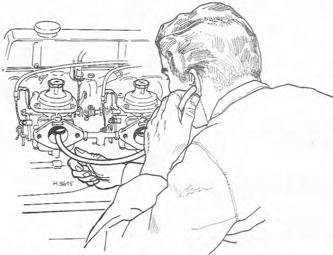
Fig. CD11 Tuning multiple carburettor set-ups. Adjust the throttle stop screws to equalise 'hiss' in each carburettor
