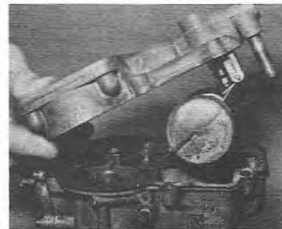
7.57 Lowering the carburettor cover assembly onto the carburettor body
