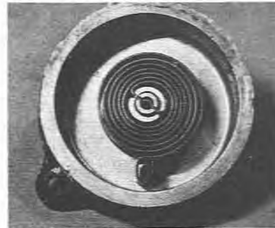
7.36 Location of the automatic choke bi-metal spring
