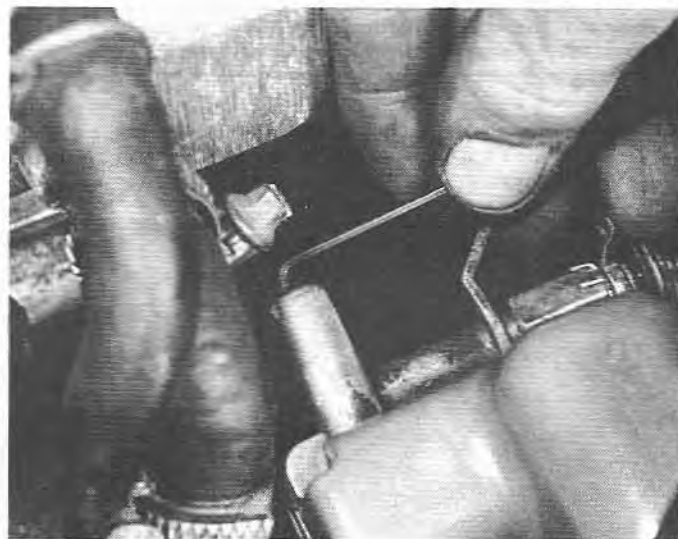
12.9 1.5 mm Allen key inserted in the FASD
