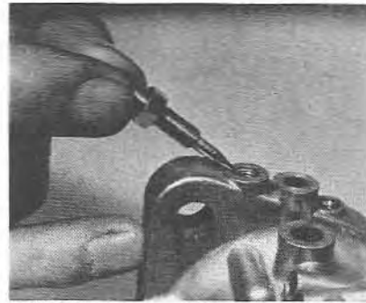
5.28 Removing an air bypass screw
