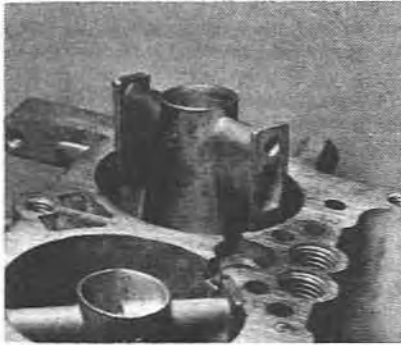
5.42 Withdrawing the primary auxiliary venturi
