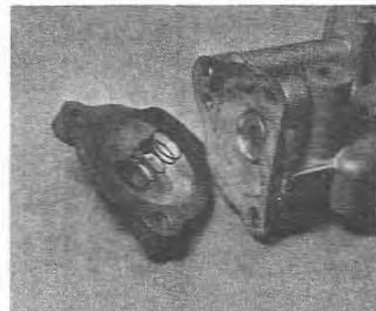
5.35 Removing the diaphragm cover (DFAV type)
