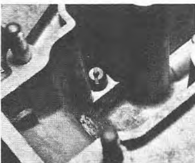
6.17 Location of an accelerator pump inlet and discharge valve (triple choke type)
