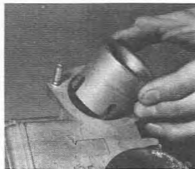
5.38 Removing a choke from the carburetor barrel
