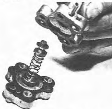
6.11a Note the strength of the spring once the cover is being removed
