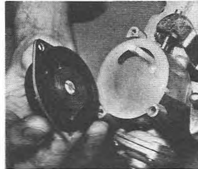
5.9a Removing the electric choke housing
