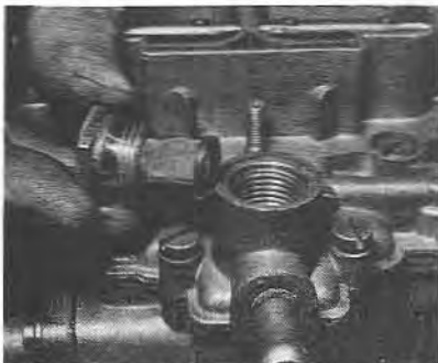
5.2 Removing the fuel filter (DFAV type)
