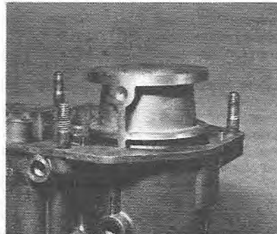
6.27a Removing a choke (triple choke type)
