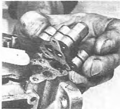
9.4 By-pass valve: watch the cleanliness here
