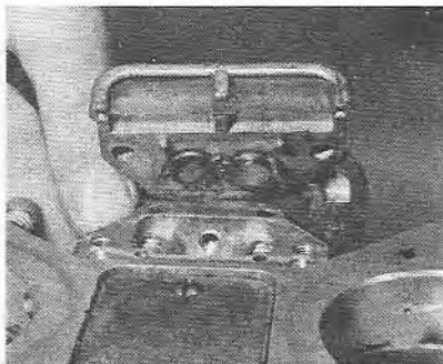
5.22 Removing the starter device, showing the locating lugs
