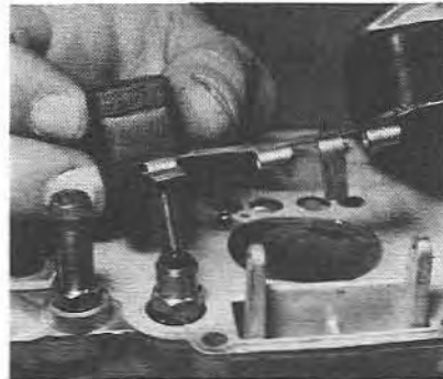
5.4b Removing the float and needle valve
