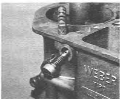
6.15a Removing an idling jet (triple choke type)
