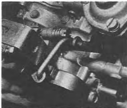
6.27 Location of the fast idle rod (DGAS type)
