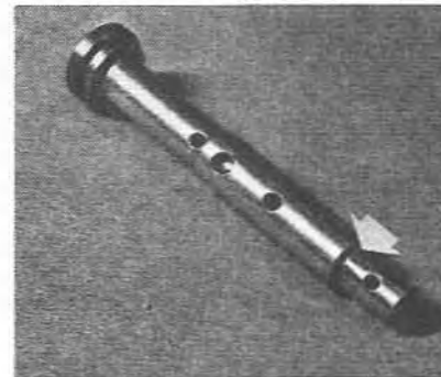
5.13b Emulsion tube size location (DFAV type)
