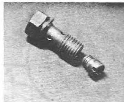
6.14b A main jet and holder (triple choke type)
