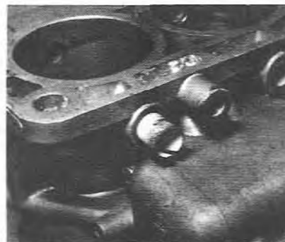
5.50b Removing a Teflon bush (DFAV type)
