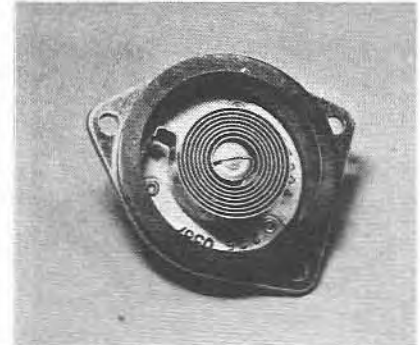
5.9b Showing the location of the electric choke bi-metallic spring
