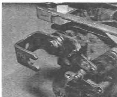
7.13 Correct assembled position of the primary sector
