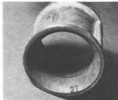
5.33 Typical choke, showing diameter identification mark
