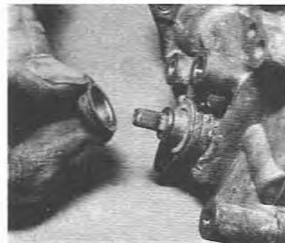
6.33b Removing the shaft cover (DGAS type)
