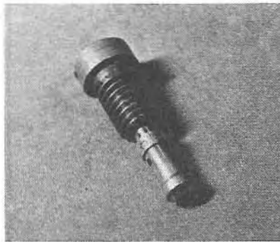
5.11c Idling jet size location (DFAV type)
