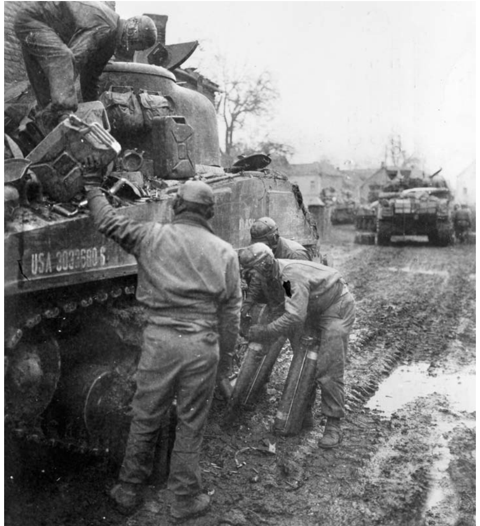
Tankers of the 2nd Armored Division use a pause in the American Army’s drive into Germany to refuel and replenish their Shermans’ ammunition supply, December 1944. The M4 tank consumed about two gallons of gasoline per mile.
