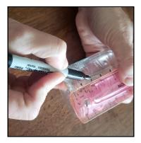
Step TWO: Use a ruler and a waterproof marker to make a scale on the bottle. You can put a strip of tape on the bottle and write on that .
