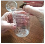
Step THREE: Place small rocks to add weight so your gauge stands up outside. For accuracy remove the rocks before reading the gauge. Put back in after.
