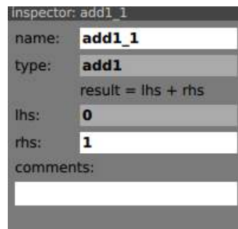
Figure A.11: The inspector showing an add1 module, a one-dimensional addition module. Only the “rhs” (right-hand-side) value is editable. “lhs” is gray and cannot be edited because it is currently connected to the output of another module.
