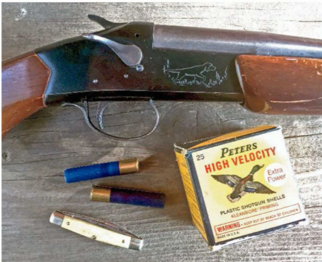
Don’t let the utilitarian engraving fool you. Payton’s 1966-vintage Stevens 940D is one solid little .410, and that side-mounted break-open lever provides an ergonomic advantage for speedy reloads—provided you’re right-handed.
