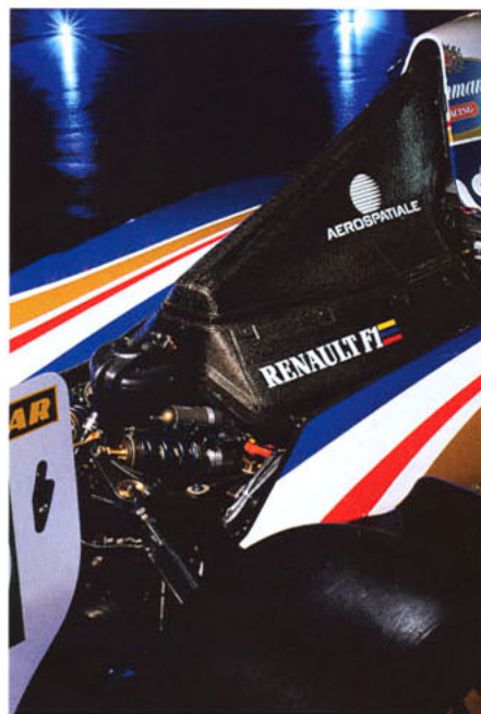
The FW19's Renault engine sat lower down in the car, giving a better centre of gravity and an eight per cent weight saving
