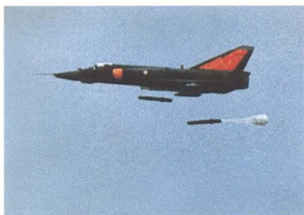
Below and right: The sequence shows the rocket-assisted anti-runway Durandal in action, from release to braking, rocket ignition, impact and detonation.
