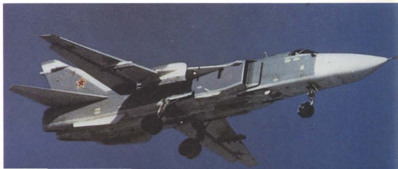
Above: Two massive drop tanks increase the range of the Su-24.
