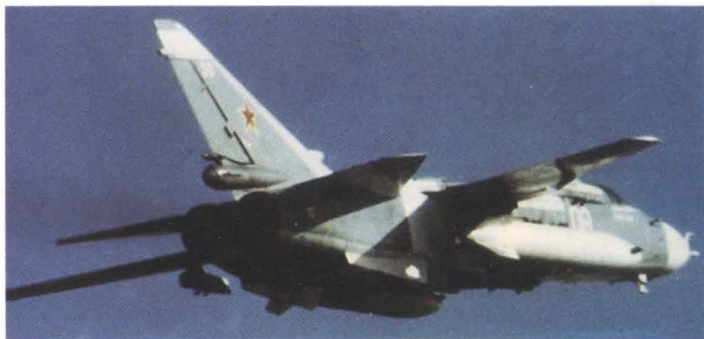
Above: Two massive drop tanks increase the range of the Su-24.
