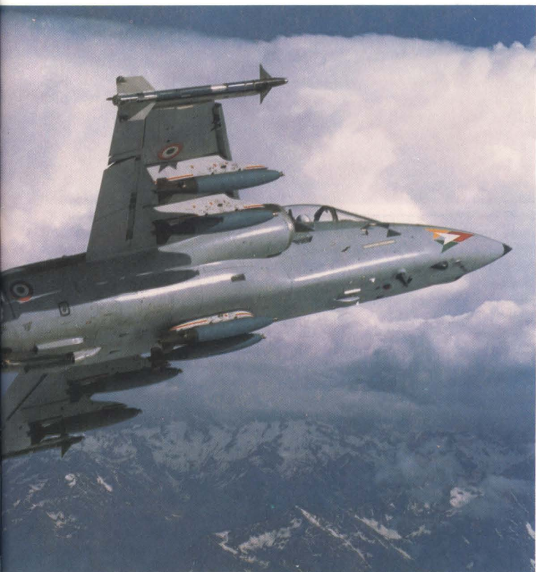
Above: The Brazilian AMX has two 30mm DEFA cannon; the Italian model has a single M61.
