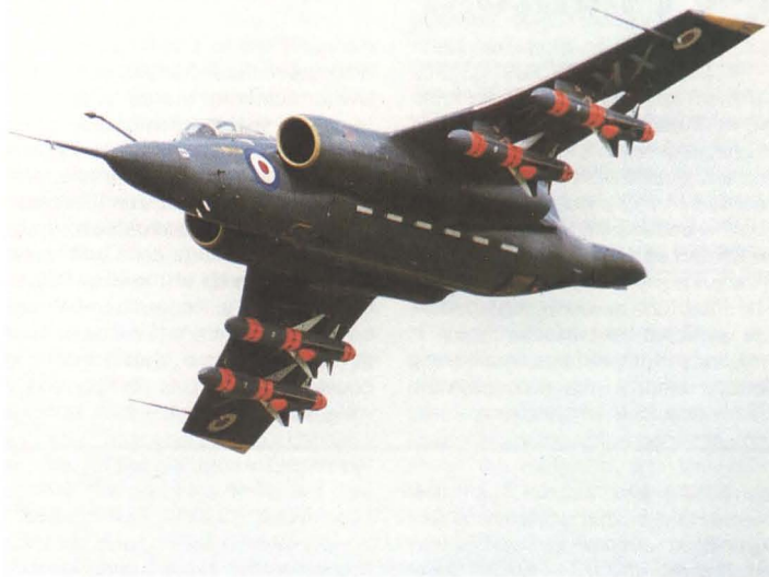
Above: The future role of the Buccaneer will be maritime strike, with Sea Eagle missiles as here as its main weapon.
