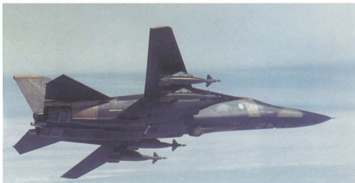
Above: An F-111A of the 366th TTW is seen over Nellis with a load of 24 Mk 82 slicks.
