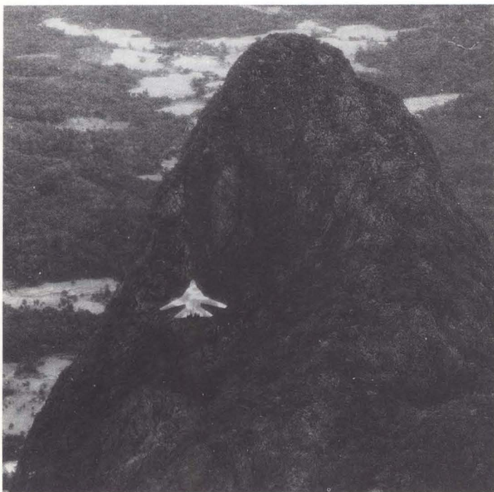
Above: An F-111 demonstrates terrain-following flight by skiing up a mountainside.
