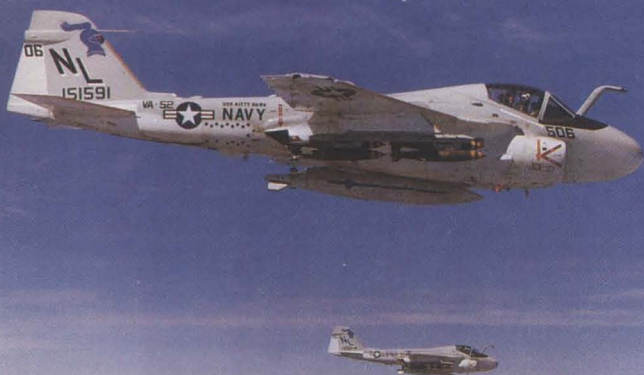
Above: The KA-6D tanker version retains an offensive capability as these VA-52 aircraft show.
