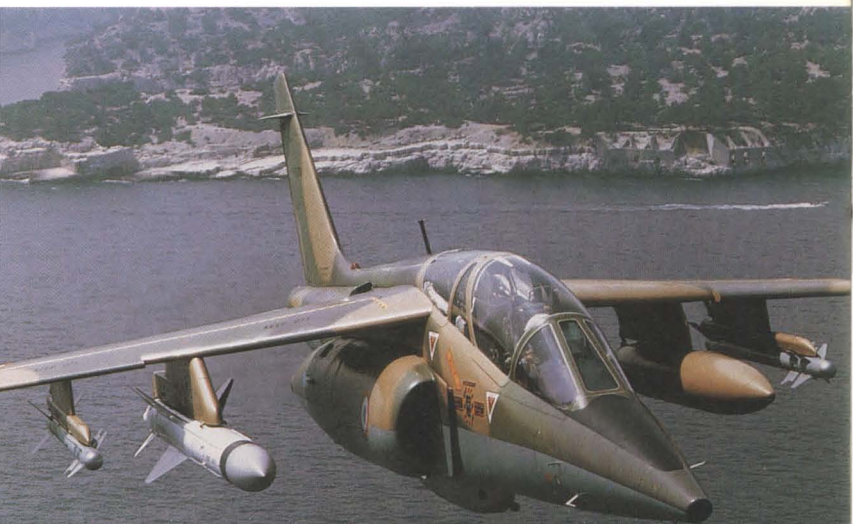
Below: The Alpha Jet NGEA has a laser ranger in the nose and an improved nav/attack system.
