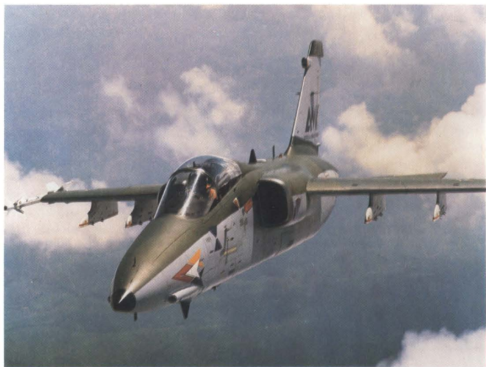
Above: The Brazilian AMX has two 30mm DEFA cannon; the Italian model has a single M61.
