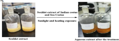
Figure 1: Colour observation for the synthesis of Silver nanoparticle; Change of colour from light cream to brownish yellow on exposure to sunlight/heating.
