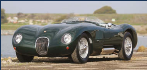
1966 Jaguar C-Type Proteus Recreation. Aluminum Bodied Recreation by Proteus. Live Rear Axle, 3.8 Liter Engine, and 4-Speed with Synchromesh and Overdrive.
