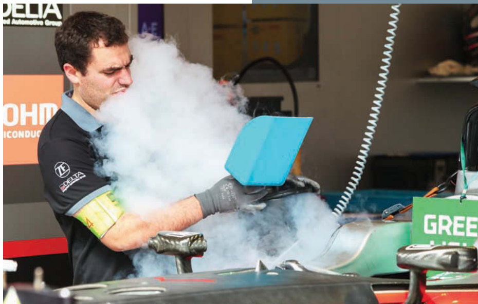
City racing: an engineer heats glue laid on cobbles which aids grip in the pits, above. Cooling the electrics with dry ice, left.
