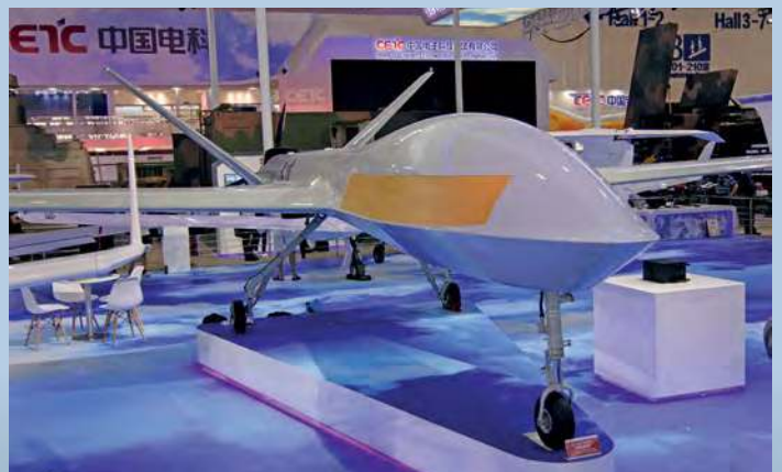
Although not visible on the mock-up, the China Electronics Technology Group Corporation JY-300 Tianshao (Sky Whistle) is designed to have sensors, including conformal active electronic scanned array radar, integrated into the airframe structure.
