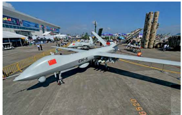
The CH-5 was presented with four AR-1B and four smaller AR-2 missiles. The smaller CH-4 is in the background.
