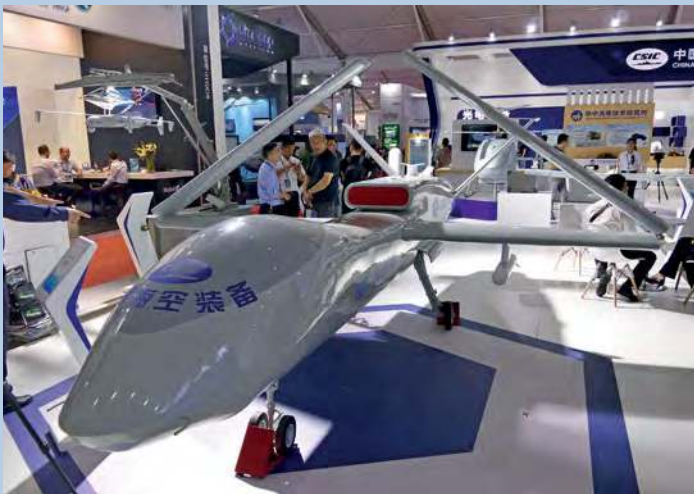
The HK-5000G armed reconnaissance UAV is intended for operation from ships and is therefore equipped with a folding wing.
