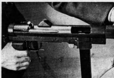
Fig 6. The gun is made safe. Notice that the cocking handle is in the safety slot.
