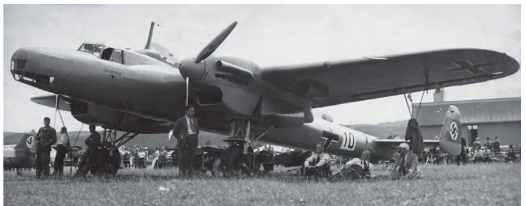
TOP: The V2, Werknummer 257 (D-AHAK), differed visibly from the V1 by virtue of the twin-tail arrangement. Both were powered by BMW VI engines. KEY COLLECTION
