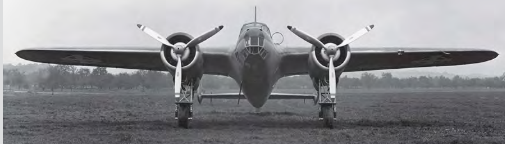
A newly produced, Gnome-Rhône 14 N1/2-powered Do 17K of the Yugoslav air arm. KEY COLLECTION
