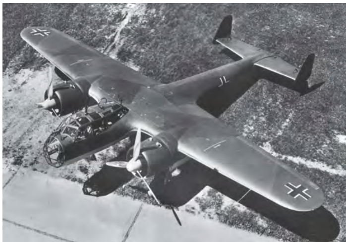
A typical production Do 17Z shows the revised forward fuselage configuration. KEY COLLECTION
