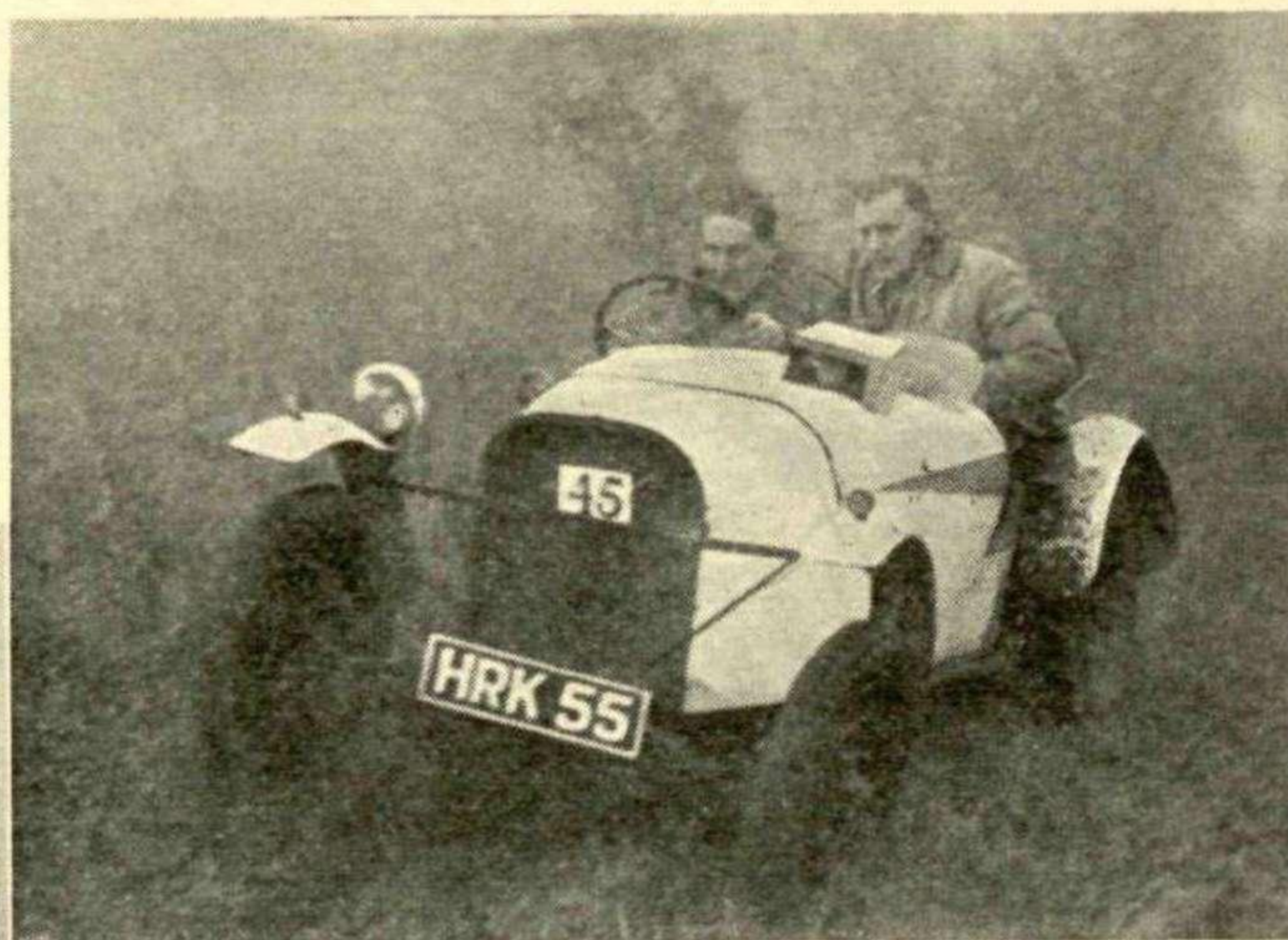
TYPICAL TRIALS SPECIAL.—A. G. Imhof's Imhof Special, runner-up in the Cottingham Trial, and winner of the Cottingham Trophy, has its blown Ford Ten engine centrally located and the rear wheels sprung independently.
