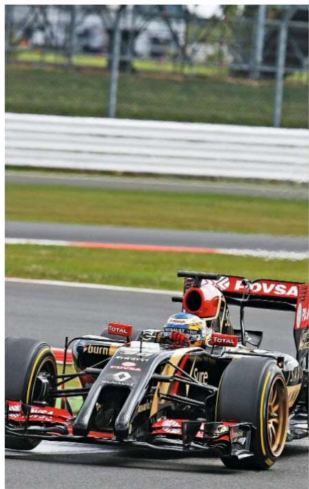
High-profile 18-inch Pirelli wheels were demonstrated by Lotus in a test at Silverstone
