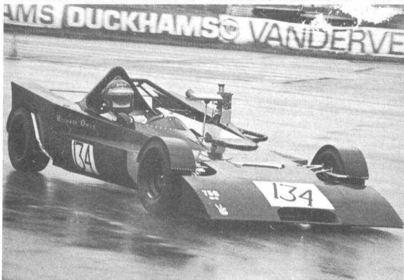
RICHARD OWEN at the wheel of Arcos 6 at Silverstone in May 1973. The car was mid-engined with the motor beside the driver and the "passenger space" in front of it. The decals on the nose of the car indicate that there were still hard feelings about the banning of Arcos 3!
