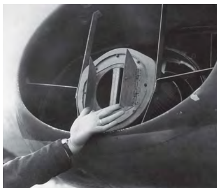
ABOVE: In a fantastic response to the dust crisis, Napier designed, built and flight-tested its deflector in one day! By midnight that day, half the company's sheet metal workers had started turning them out and within a week the whole Typhoon force had been equipped.
