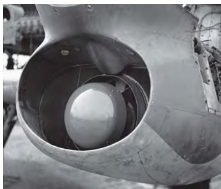
ABOVE: In a fantastic response to the dust crisis, Napier designed, built and flight-tested its deflector in one day! By midnight that day, half the company's sheet metal workers had started turning them out and within a week the whole Typhoon force had been equipped.
