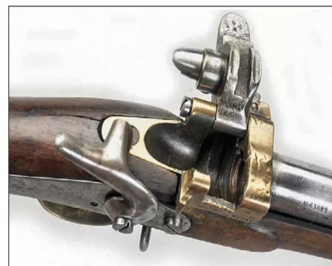
A close up of the Krnka's hinged breech system.
