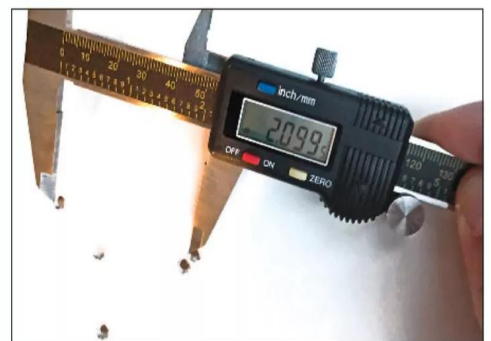
The best group at 50 yards for 5.56 came from Winchester's USA Ready 62-grain OT. It measured in at 2.10 inches and 1.59 without the flyer.
