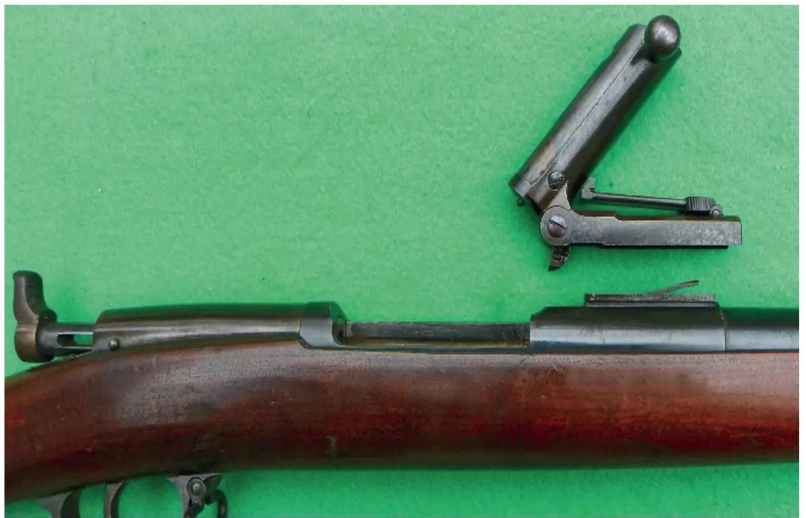
The obr. 1868g was based upon a “trapdoor” type breech which automatically ejected the spent cartridge case. Note the large, curved cocking piece on the end of the striker. (Courtesy Nick Stanev)
