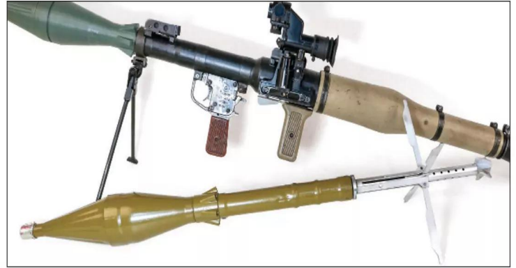
The geometry of the RPG-7 round causes it to track counterintuitively into the wind when fired in a crosswind.
