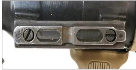
The optics rail on the side of the RPG-7 is Combloc standard.
