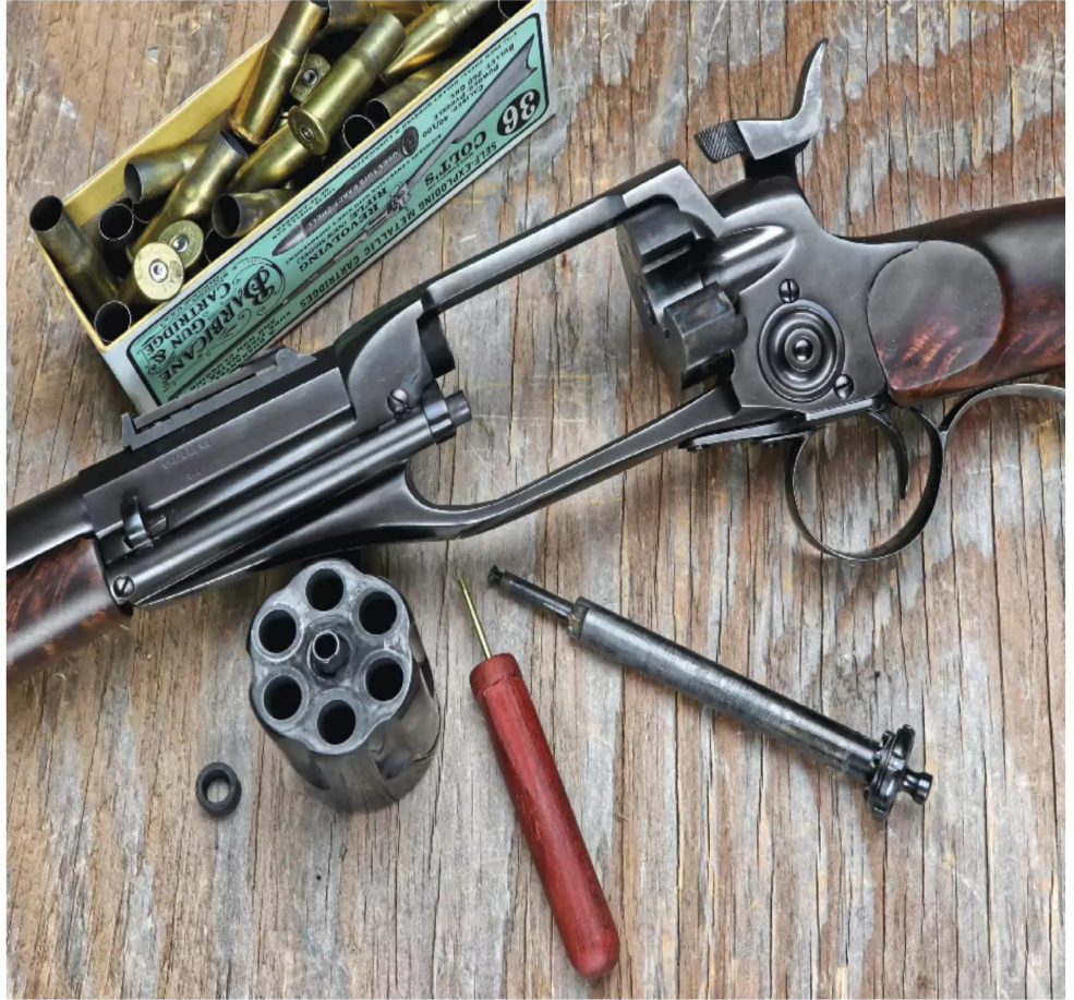
Disassembly is easy, but requires a little tool. The once large, external cylinder pin plunger (just visible under its retaining screw in the frame) is now flush and under the ejector rod housing, but has a little window for the tool. Half cock the rifle, ensure the cylinder is unloaded, push in the pin, and withdraw the cylinder pin. Take the cylinder out of the window, roll up your sleeves and go to work. No other disassembly is required. Note the external endshake bushing to the left of the cylinder. Normally you'd want something like that captive, but there was no good way to do so. Note also how small the cylinder pin is where it exits the cylinder and enters the frame. It is smaller in diameter than a Colt SAA's cylinder pin, and another reason the gun shouldn't be fired with high-pressure loads.
