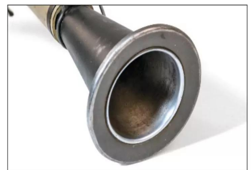
The interior of the RPG-7 tube is either hard chrome-plated or stainless for wear and corrosion resistance.
