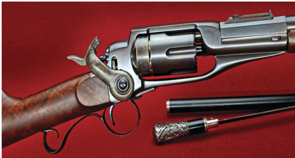
The hand is mounted to the hammer and operates through a large window in the action. This opening is mostly protected from debris by the hammer. It apparently never caused much of a problem, or at least never as much as cap debris did in most percussion arms. The advent of the metallic cartridge obviated such concerns forever.
