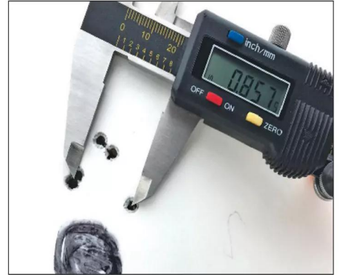
The smallest 5.56 group at 25 yards came from Winchester's USA Ready 62-grain Open Tip at .86 of an inch, and without the flyer only .67 of an inch — a tie with Black Hills' best group without its flyer.
