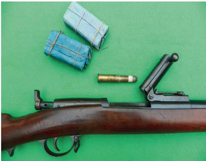
The obr. 1868g was based upon a “trapdoor” type breech which automatically ejected the spent cartridge case. Note the large, curved cocking piece on the end of the striker. (Courtesy Nick Stanev)
