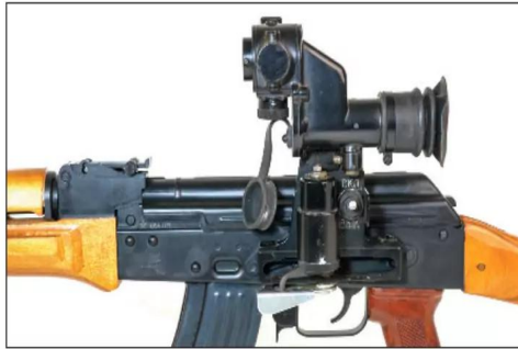
The PGO-7 optic is actually a seamless fit on the side of this AKM. Though the resulting eye relief is awful, the #2 range line makes a decent 100-meter zero on an AKM.
