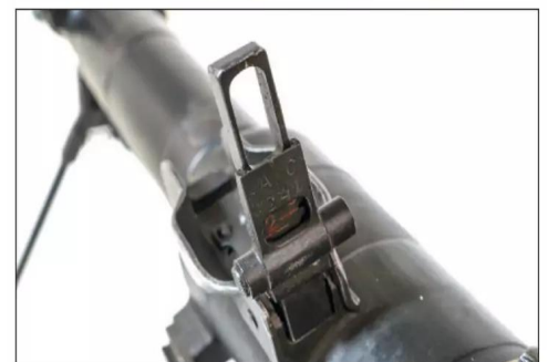
The folding iron sights are simple but effective.
