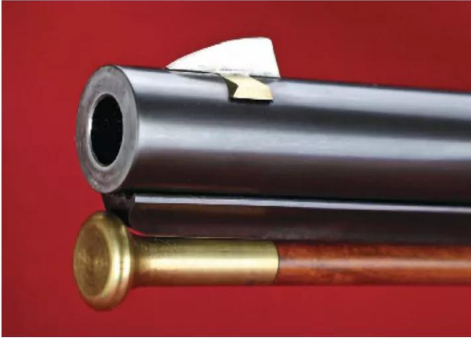
A Ted Cash German silver front sight with a 0.050-inch blade was filed to a rakish shape to zero the rifle.
