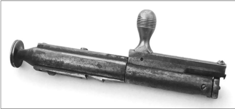
The obr. 1870g used a two-piece bolt with a distinctive short bolt handle and a large cocking piece.
