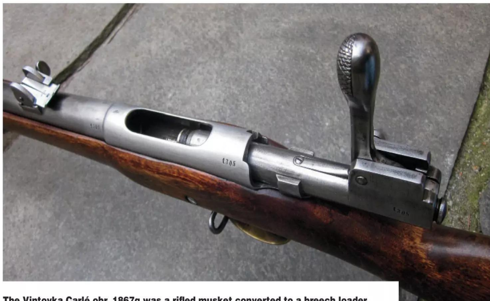
The Vintovka Carlé obr. 1867g was a rifled musket converted to a breech loader.
