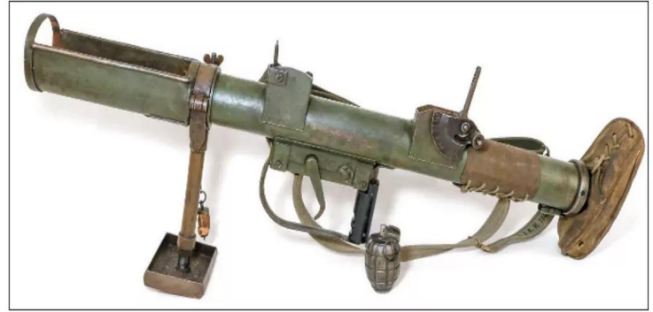
The WW2-vintage British PIAT (Projector, Infantry, Anti-Tank) was a beast of a thing that weighed some 32 pounds. Technically a spigot mortar firing shaped charge warheads, the PIAT accounted for 7% of all the German tanks destroyed by Commonwealth forces during the Normandy campaign. By comparison, aircraft of all types accounted for 6%.
