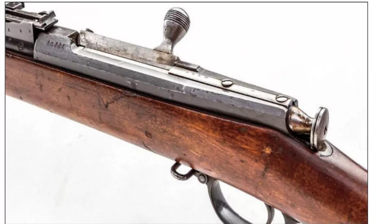
Its most distinctive feature of the obr. 1870g was a bolt handle that stuck up at a 45° angle when the bolt was closed.
