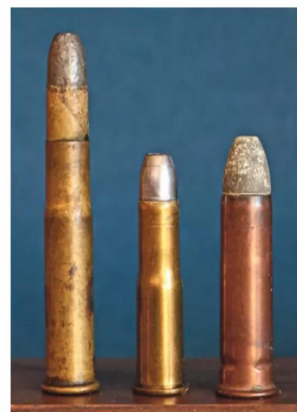
The .40-50 SBN (middle) was one of our first centerfire cartridges and quite successful against thin-skinned game. So successful, many other manufacturers duplicated its ballistics culminating in the .40-65 Winchester, from whence the bullet for these loads comes. The .40-50 is flanked by two cartridges stealing its limelight. The immensely popular .44-77 Sharps & Remington (left) was widely used in the early buffalo hunting era as well as one of our first premier long-range shooting rounds. The .50-70 Gov't (right), was also quite popular for buffalo hunting, and is shown in its copper-cased, inside primed military issue.
