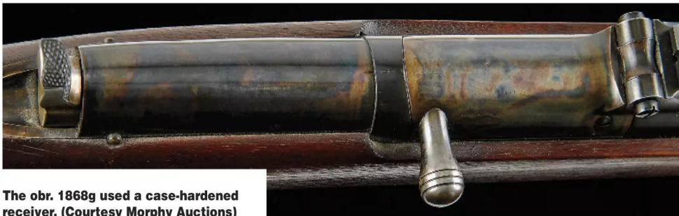
The obr. 1868g was based upon a “trapdoor” type breech which automatically ejected the spent cartridge case. Note the large, curved cocking piece on the end of the striker. (Courtesy Nick Stanev)
