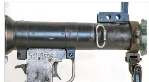
There was a dedicated sling with dual snap hooks designed for the launcher.
