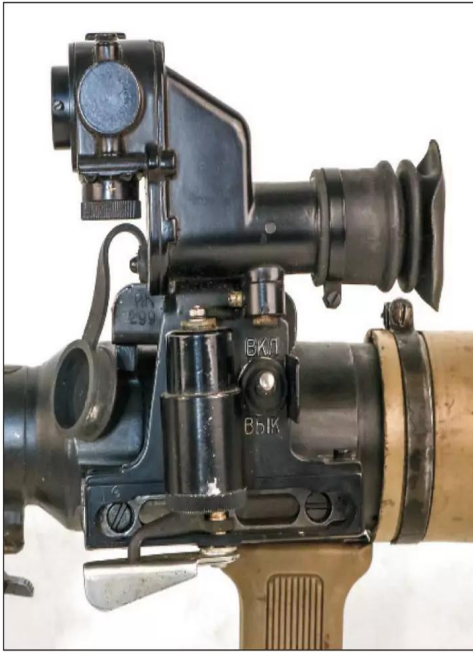
The PGO-7 optical sight features a battery-powered illuminated reticle and 2.7X magnification. The offset nature of the design is so that the line of sight can peek around the warhead.
