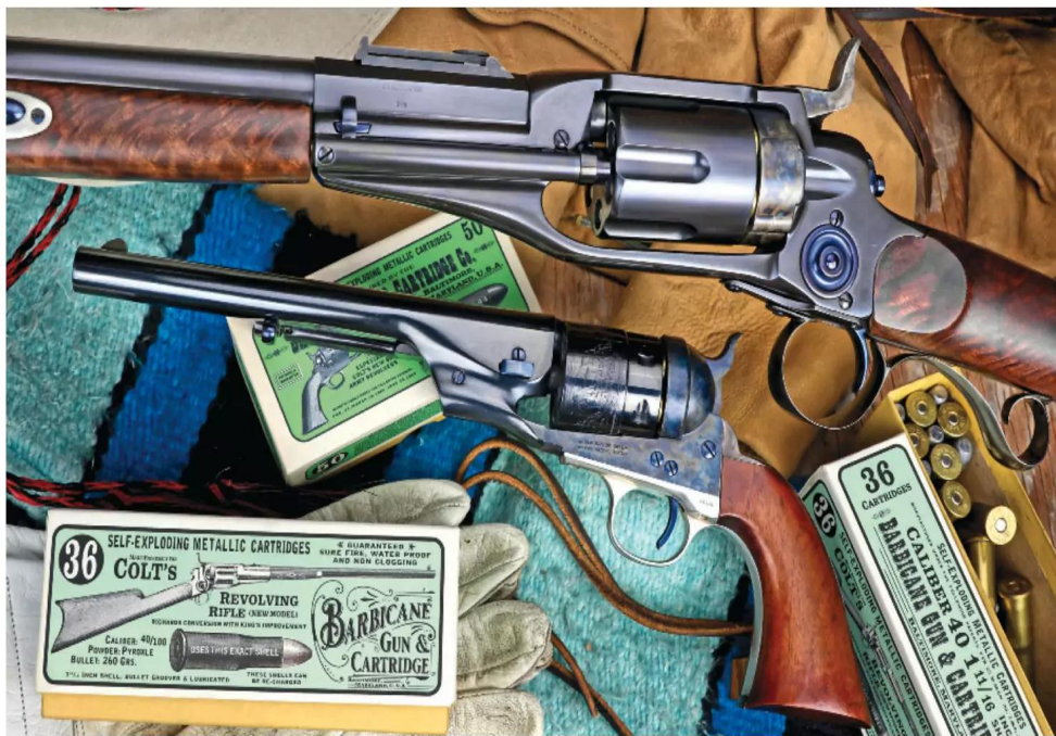
A rifle deserves a suitable companion handgun, and the big Colt rifle is paired with a Cimarron copy of the Colt 1860 Richards/Mason conversion in .44 Colt. The .44 Colt and .40-50 SBN are two of America's earliest centerfire cartridges.
