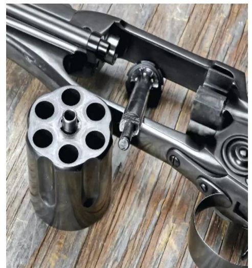
The "Transporter" (as Palmetto calls it) at the front of the cylinder ensures chamber/barrel alignment with the bolt locking notches on the cylinder pin. Once aligned, the transporter is secured by twin pins on either side of the cylinder. The front of the cylinder pin (shown next to the cylinder facing from the frame window) has twin lugs engaging corresponding recesses in the transporter to rotate the cylinder. The two have to be in perfect alignment at the very front and very rear for the system to work.
