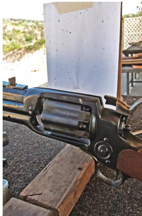
A paper shield was erected to see why the percussion gun's accuracy was so execrable, and the shooter so annoyed. A "transporter" misalignment of cylinder-to-barrel caused bullet debris to eject forcibly out the right. The left-hand shield showed less than half this amount of detritus, some of which penetrated the paper on the right. Luckily, the other shooting benches were unoccupied. Wear shooting glasses at the range, just in case the author shows up with some ill-mannered contraption.
