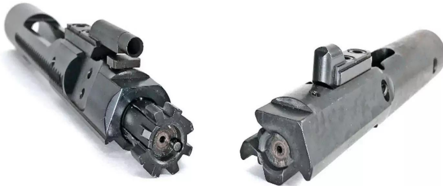
Comparison of the bolt assemblies for the Hellfire 5.56 (LEFT) and Hellfire 9MM (RIGHT). Note the lack of a separate bolt assembly on the 9mm carrier, as well as the lack of gas key, as this firearm is blowback-operated.
