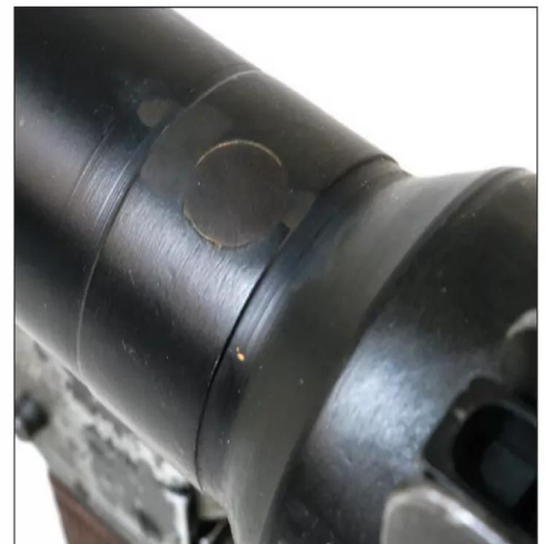
Part of the demilling process involves welding a steel bar across the interior of the tube. I touched up the weld spot with a little cold blue.
