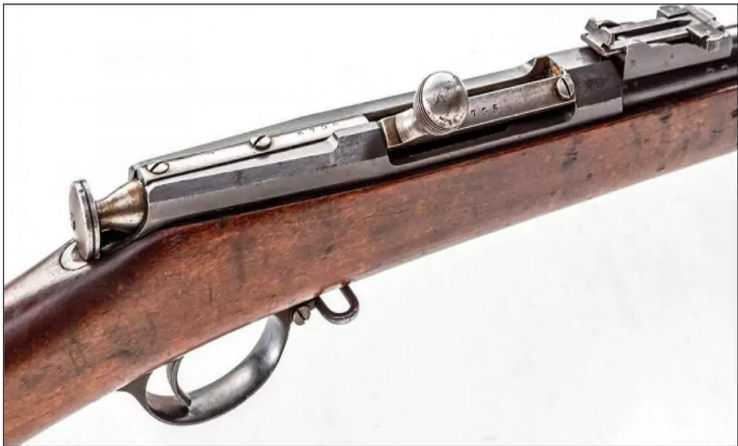
Its most distinctive feature of the obr. 1870g was a bolt handle that stuck up at a 45° angle when the bolt was closed.
