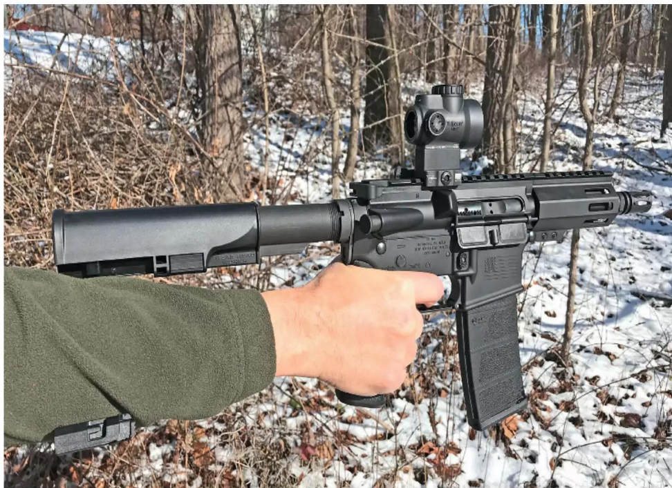
The new BATFE-approved Tailhook MOD2 is as comfortable as the original model and shifts the firearm's weight from the wrist (relieving stress) to the forearm. It also incorporates a unique track system, which allows the brace to be quickly adjusted within BATFE regulations.
