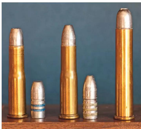
The bullets developing the best performance in the rifle include a commercial hardcast 275-grain plain-base bullet (left pair), and a home cast 320-grain bullet dropped from 30:1 alloy in the RCBS 40-300 CSA mold and SPG lubed (middle pair). Both are sized .406 inch. To the right is a .45-70-405 Gov't for comparison.
