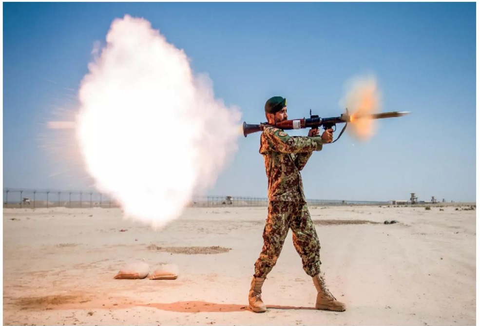
The RPG-7 produces some ample chaos out its butt. Like all recoilless weapons of this sort, it is imperative that you clear your backblast area before firing. (DOD photo — SSG Ezekiel Kitandwe)
