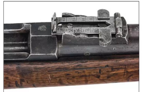
The rear sight of the obr. 1870g was adjustable from 200 to 1,500 arshini. Note the notch on the right side of the sight slider which was used with a stud on the front barrel band allowing adjustment up to 2250 arshini.
