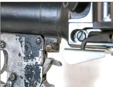
The manual hammer is designed to be cocked with the firing thumb.
