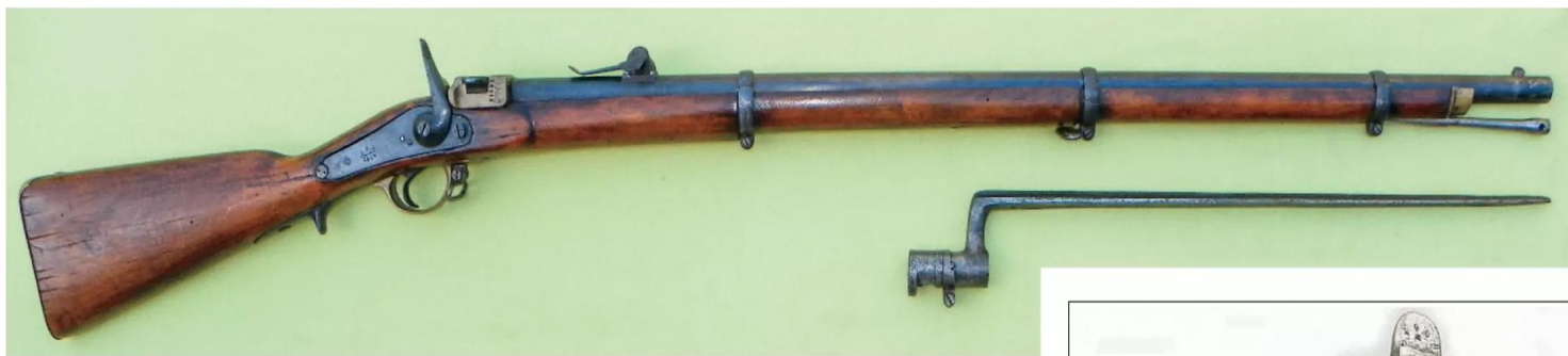
The Vintovka Krnka obr. 1867g was the Russian army's first metallic cartridge, breech loading rifle. (Nick Stanev photo)
