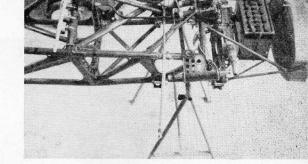
THE BATTERY is carried in the front of the car (above). Rack and pinion steering is employed. REAR DISC BRAKES are mounted inboard (below). A six-speed A six-speed Colotti gearbox is used.
