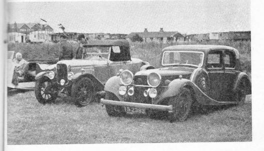
tourer. An example with this coachwork tried some twenty years after construction was found to have surprisingly good handling, not in accord with the reputation of the early Speed 20, and was still capable of 0-60 in just over 26 seconds; an indicated 80 m.p.h. was obtained without mechanical stress and fuel consumption worked out at 17 m.p.g. A Speed 20, suitable for restoration, can now be purchased for well under £100.
