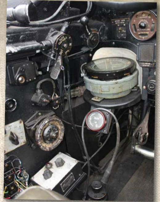
BELOW LEFT: To the right of the pilot's seat are the undercarriage selector lever and safety bolt, painted red, and beyond them the aileron, rudder and elevator trim wheels. The undercarriage control safety bolt prevents unintentional operation of the landing gear. Note the proximity of the Air Bomber's position. (HMP)
