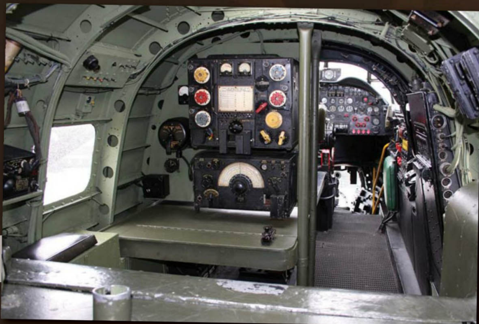
RIGHT: The Wireless Operator's position in Just Jane . Note the top of the front wing spar in the foreground. (HMP)
