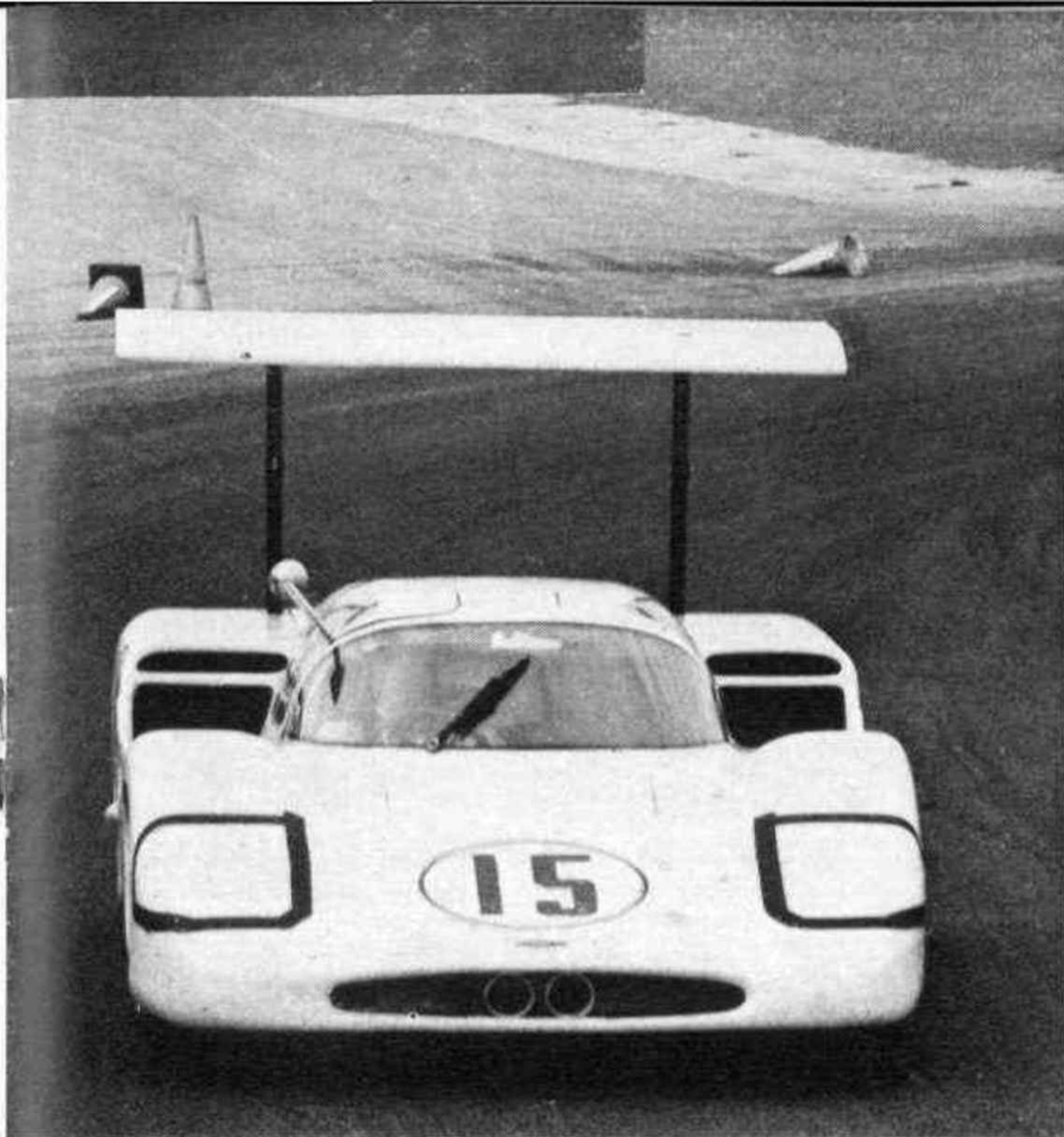
CHAPARRAL 2F.—The latest car turning onto the banking at the point where it skidded into the retaining wall after three hours. For this race the overhead wing spoiler is at a fixed angle. Double intakes beside the cockpit duct air to the carburetters, radiators and brakes.
