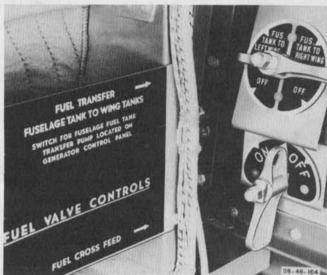
Figure 26—Fuel Transfer and Cross-feed Controls
