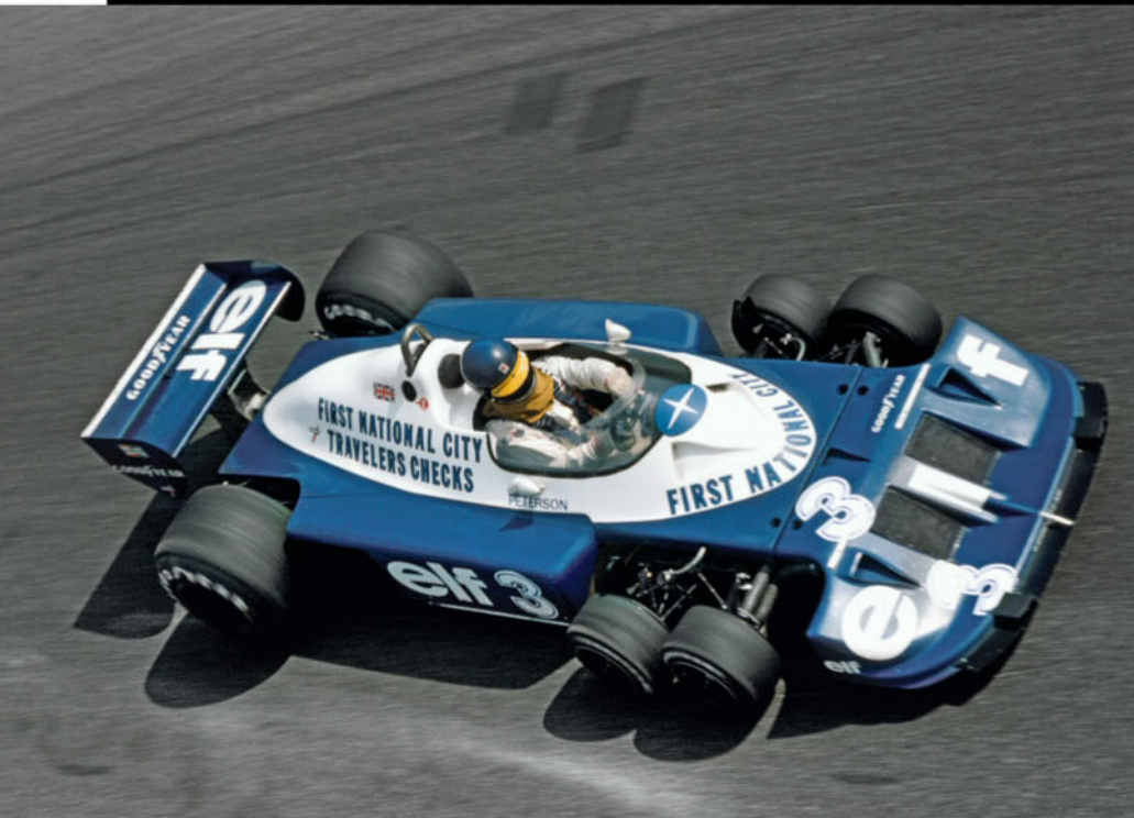
The six-wheel P34, with its nine-inch front tyres
