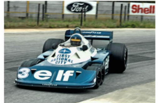
The six-wheel P34, with its nine-inch front tyres
