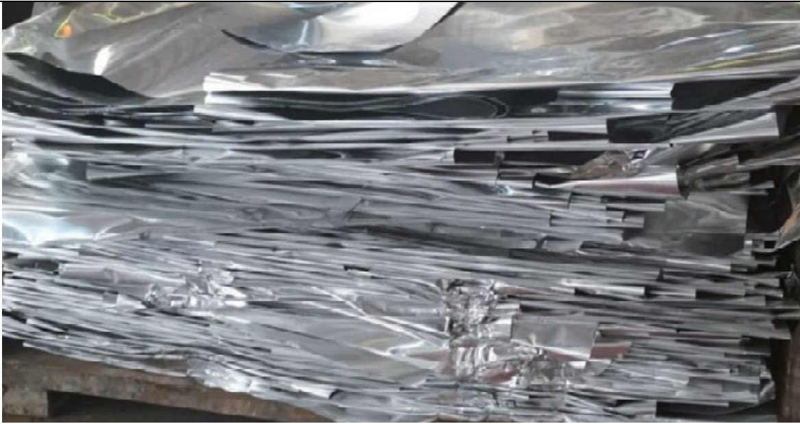
Figure A.3 New clean printing plate base
