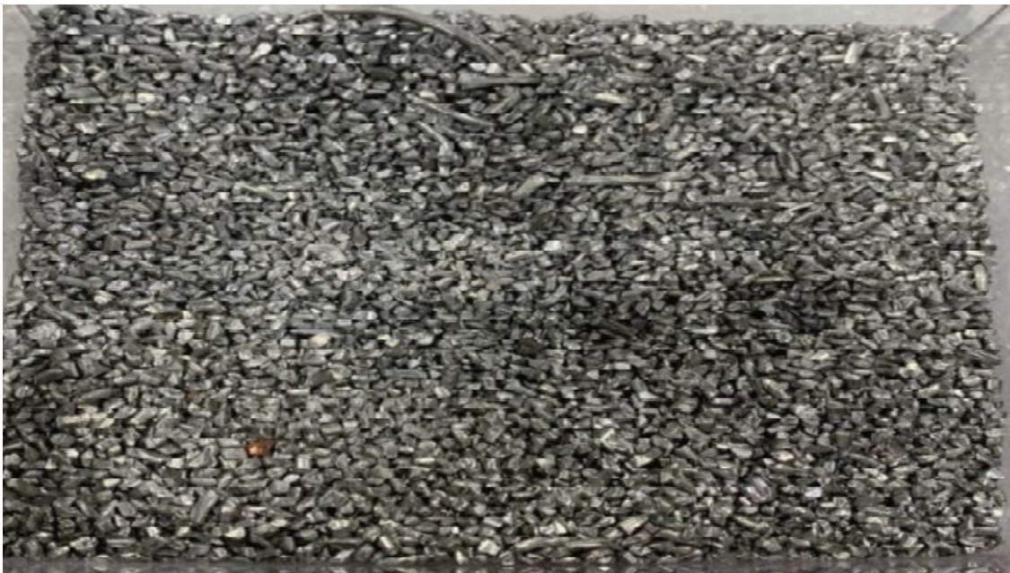
Figure A.6 Electrical aluminum particles
