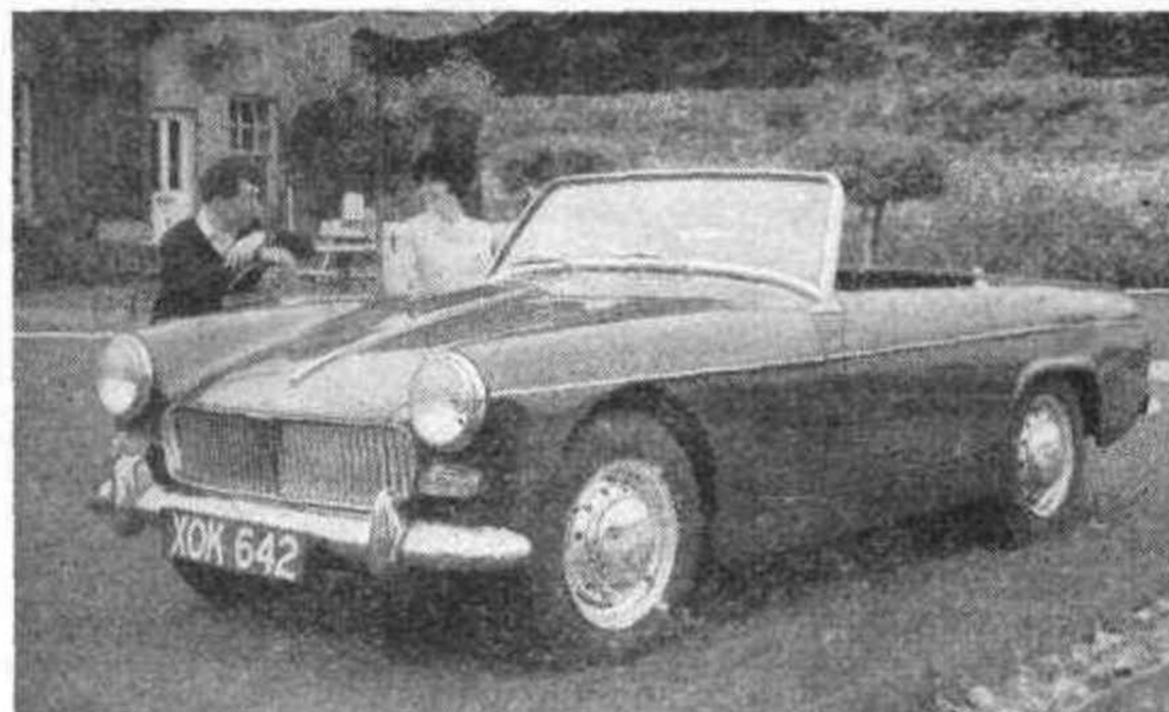
JUST RELEASED. —This is the new 948-c.c. M.G. Midget, for which 46.4 b.h.p. at 5,500 r.p.m. is claimed. We wonder how it compares for quality, appearance and European price with the Innocenti 950 ? We hear that a new Mk. II Austin Healey Sprite has also been announced, which B.M.C. refer to as "the safest sports car in the world." They claim for it "90 m.p.h. with ease and 0-60 m.p.h. in 17.4 seconds" but the first independent road-test report we read quotes a top speed of 85½ m.p.h. and 0-60 in 19.8 seconds. We wouldn't know—MOTOR SPORT wasn't invited to the party !
