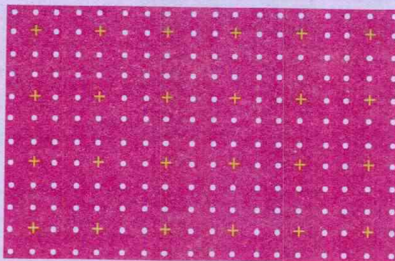
Fig. 4.2 A schematic diagram of Copper wire showing its positive nuclei (+) embedded in sea of free electrons (o) making 'Metallic Bonding'
