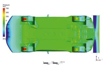
Figure 8: The pressure was negative under the 2017 baseline racecar's splitter
