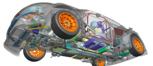
Prodrive used a master CAD model to analyse five different engine and drivetrain layout concepts. It decided on a longitudinal layout as opposed to transverse as this allowed the CoG to be as low as possible as well as giving the desired mass distribution
