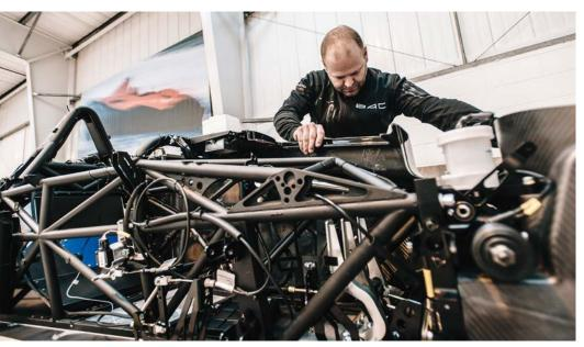
The car uses a spaceframe rather than a carbon monocoque. BAC says this provides good torsional rigidity at a lower cost
