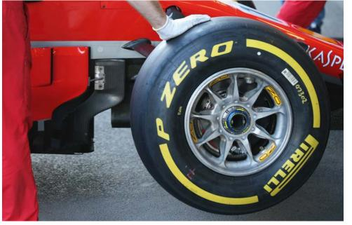
From 2019 the practice of allowing air to escape via ducts in the centre of the front axle (known as 'blown nuts') is banned
