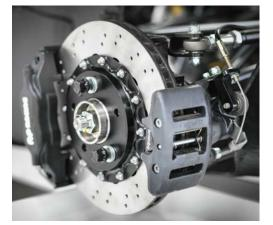
The brakes are race specification, featuring 295mm ventilated discs clamped by AP Racing calipers. Hi-tech ceramic brakes for the BAC Mono have been developed by Surface Transforms
