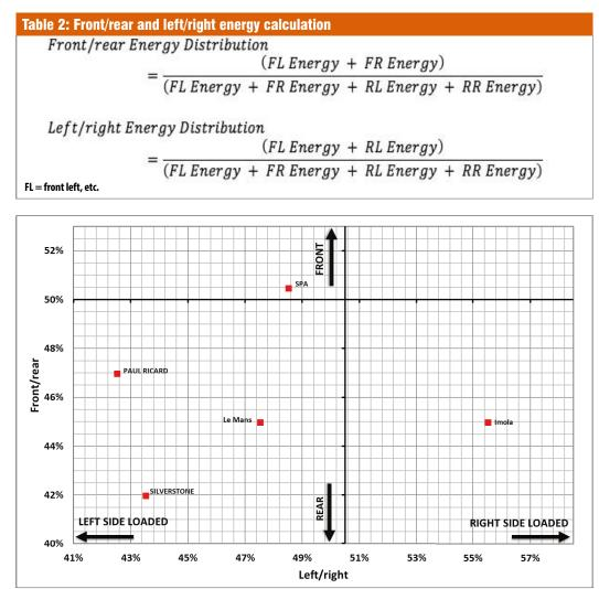
Figure 5: This gives us a visual reference as to how the sliding energy is distributed between tyres at different tracks
