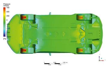
Figure 3: Suction over bonnet and roof is offset by pressure on splitter and rear deck
