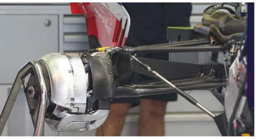
The rear suspension on the car is pullrod with torsion bars. Note how the driveshaft runs right through the lower wishbone
