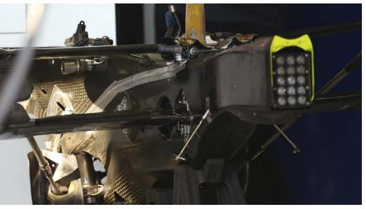
The carbon fibre gearbox had to be specifically designed for the Honda PU, although it is similar in concept to last year
