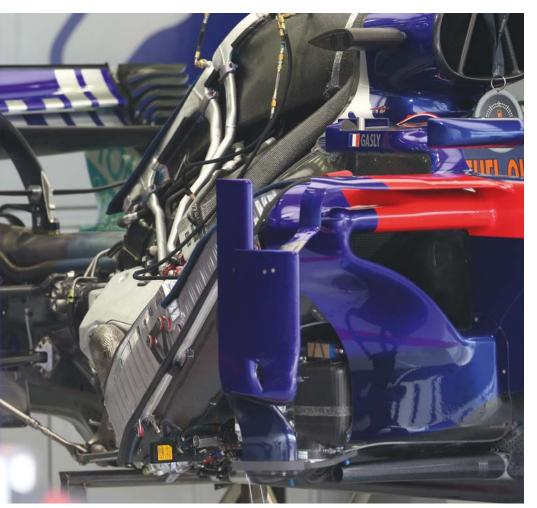
The cooling layout is similar to last year's STR12, despite the change of power unit. Note the cooler on the car's centreline
