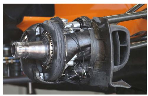
The size and position of brake ducts has been more tightly defined in the 2019 regulations and solutions such as this on the McLaren will not be allowed. Teams are highly likely to try to exploit the shape of the scoop to recapture losses in this area
