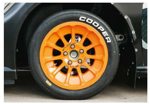
Inboard brakes allowed for a completely different wheel design, but manufacturers didn't have the tools to make it so Prodrive partnered with OZ to develop a bespoke wheel that's said to be light and also good for tyre pressure control
