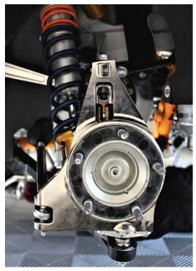
The wheel hubs do not need to accommodate brake calipers, discs or pads because of the Megane's clever inboard braking system
