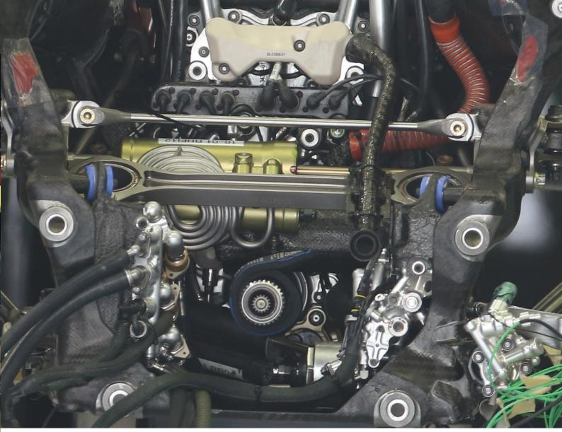
Rear torsion bars and other inboard suspension parts are located within the bellhousing; note transverse mounted dampers. Suspension system is smaller and lighter than in 2017
