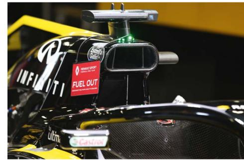
A large portion of the cooling package is in the centre of the racecar but the introduction of the Halo was an unexpected complication as an additional cooling duct had by then been mounted behind the driver's head
