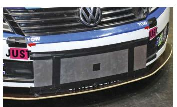
Blanking of the front ducts completely resulted in a modest decrease in the car's drag
