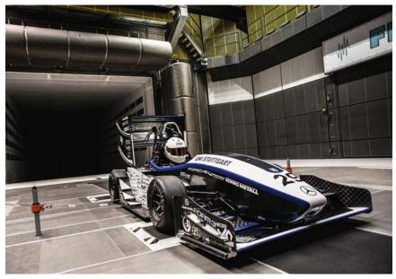
Wind tunnels provide an excellent validation tool for CFD and are still very widely used. Even Formula Student teams might test their cars in a wind tunnel – here the Stuttgart FS team's car is shown in the FKFS facility
