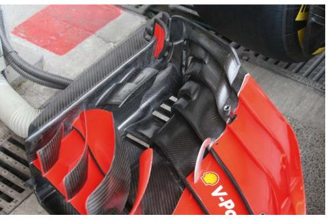
At the heart of the new regulations is a desire to do away with the vastly complex front wing arrangements that are a part and parcel of F1 (as seen here on the Ferrari) and the out-wash they are designed to create
