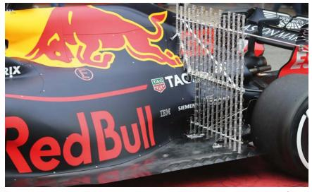
Though heavily restricted in F1 track testing is also an essential tool for optimising aero performance. Often Formula 1 teams will use pressure rakes to measure the static pressure of airflow coming on to the rear wing
