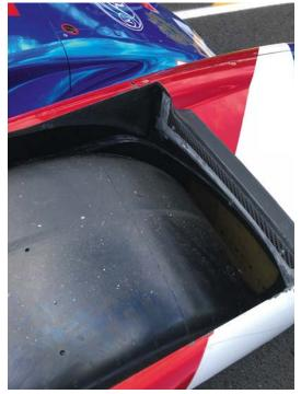
Dallara redesigned the front wheel arch on its BR1 following a spectacular Spa flip. The larger hole added a little drag but it also reduced the impact of rubber build-up on the downforce
