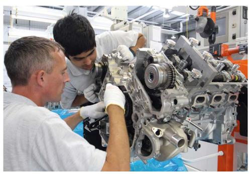
Each of the stations on the production line is equipped with an HMI screen which walks the Ricardo technician through the required tasks; from the tool that they should be using for the job to how much torque should be applied to each of the bolts
