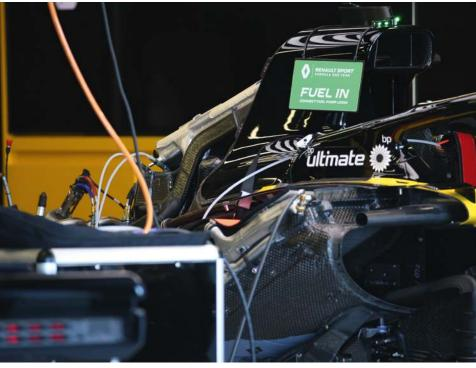
Relocating the coolers to the centre of the car has helped to reduce the sidepod volume, which is all part of a concerted effort by the design team to force higher energy air to the rear of the car to work the diffuser harder
