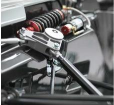
The suspension is a fully adjustable pushrod system with Sachs dampers. Such adjustability is crucial on a car that can be used both on the road and on the race track
