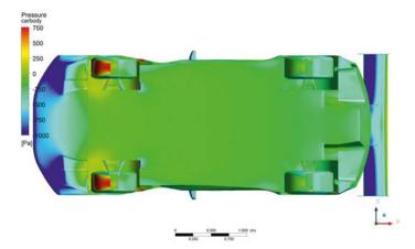
Figure 16: The modified end fences and angled walls improved the dual-height diffuser
