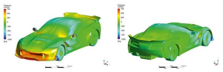
Figures 1 and 2: The pressure highs and lows on the road model of the Corvette go some way to revealing the sources of drag, lift and downforce in the car
