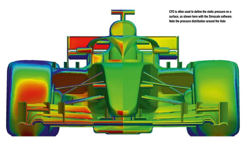
n recent years we have constantly been told computational fluid dynamics (CFD) would revolutionise the aerodynamic development of racecars. This has indeed been the case, supported by the relentless development in computational technology and modelling techniques. However, CFD has not yet advanced enough to replace wind tunnels entirely, as was at one time forecasted.
