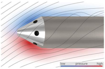
Diagram showing the air pressure differences around the point of a Pitot tube. These have multiple holes so that the total and static pressure can be measured as well as the angle of attack and the flow velocity
