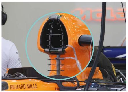
Pressure rakes are often made up of a series of Kiel probes which are designed to measure the total pressure of the flow at non-zero angles of attack. F1 teams tend to use FP1 for aerodynamic testing at the race circuit
