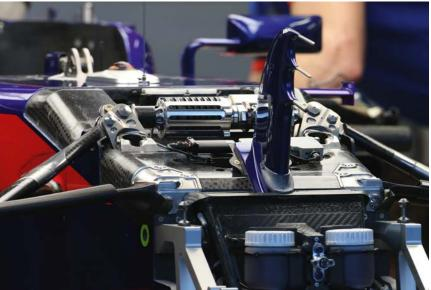
Front suspension showing the third element damper. The front of the car is very similar to last year's STR12
