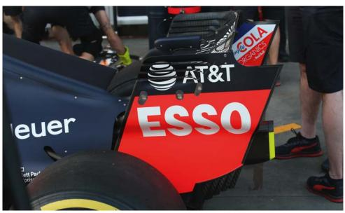
The canted back shape of the rear wing endplates will remain but the wing itself will be bigger to allow for a larger DRS slot
