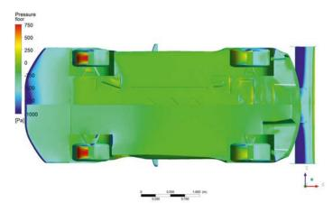
Figure 10: Underside pressures changed to those shown in the lower half of this image
