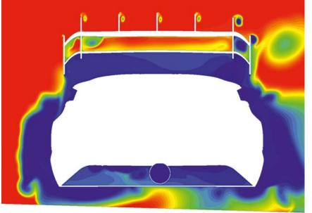
Much of Prodrive's CFD analysis for the Megane was focused on maintaining the downforce from the rear wing during the high yaw angles experienced during a rallycross race, when the cars are very often sliding
