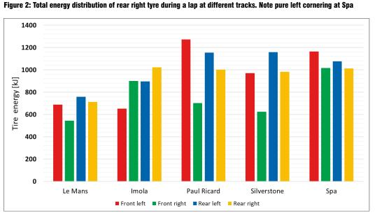
Figure 3: Total tyre energy in each wheel at different tracks. Note that at Imola front and rear right tyres are used more
