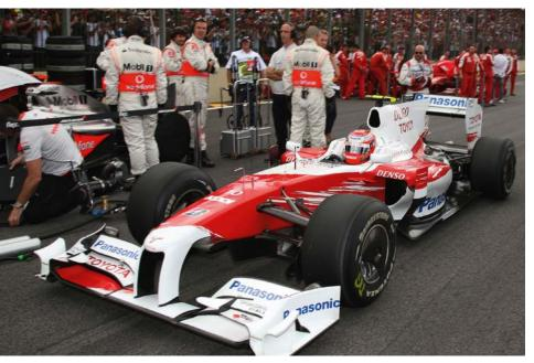
Out-washing front wing endplates first appeared in 2009 (seen here on Toyota's TF109) and quickly proved to be detrimental to the quality of the racing. Many believe the problem should have been addressed back then
