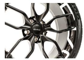
The Mono uses a carbon fibre/aluminium hybrid wheel to help save weight. The tyres have been specially developed by Kumho chassis is not as fragile as carbon and is much easier to repair. The chassis structure is said to be very robust for its light weight and torsional stiffness is exactly where it needs to be.
