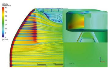
Figure 13: Stall could be seen in the outer section of the first front diffusers we tried
