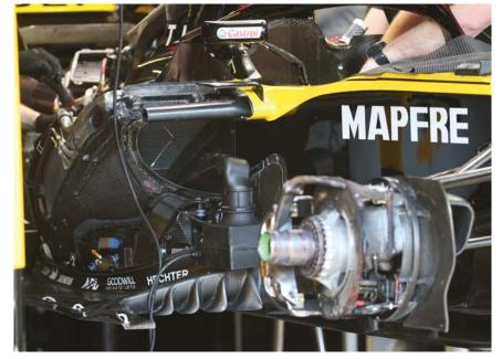
Sidepods with the bodywork removed. Renault has adopted the short sidepod style pioneered by Ferrari rather than opting for the lighter conventional layout. Brake calipers are by Brembo, master cylinders by AP Racing
