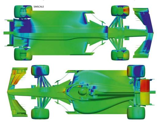
CFD is predominantly used to understand the internal and local flow field properties and is ideal for detailed aero work
