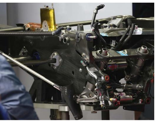
The internal rear suspension layout had to be changed due to the differences between the Honda and Renault power units
