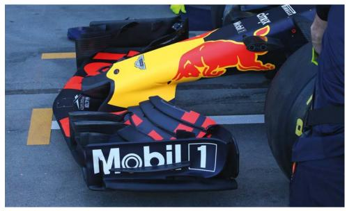
With a view to restricting out-washing devices, as seen on the Red Bull, front endplate design has been drastically restricted
