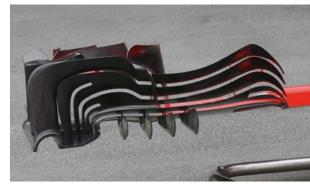
Only two strakes on each part of the underside of the front wing will be permitted when the new rules come into force. This year some teams have been using as many as four (Ferrari pictured)
