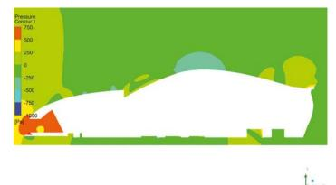
Figure 4: Pressure was actually raised under most of the road model's splitter
