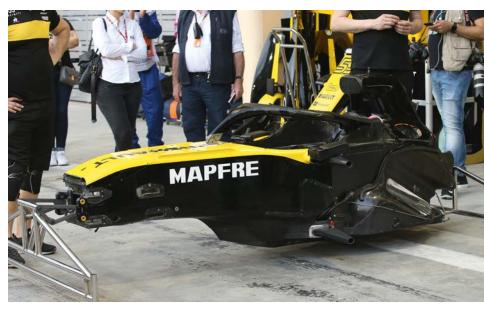
RS18 monocoque stripped down to its bare essentials. Weight reduction in the chassis was a major element of the car's design philosophy but Renault says this is still marginal and it has struggled to hit the weight limit
