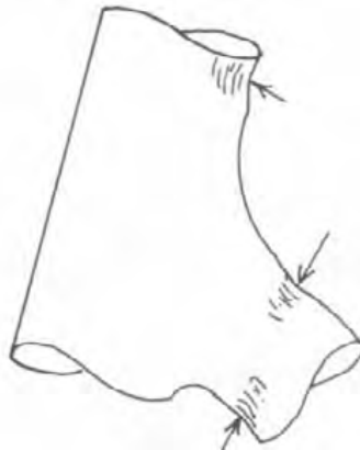
BADLY UNDERCUT JOINT
