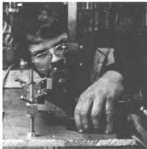
FIG #110 Set the fork jig for the correct amount of rake. To get the right height for the top of the axle add up the following values: 1-Height of centerline of column above the surface of the jig, 2-Amount of rake desired, 3-Radius of axle. This will give the reading to set the vernier height gauge at. (See Step IV-33)
