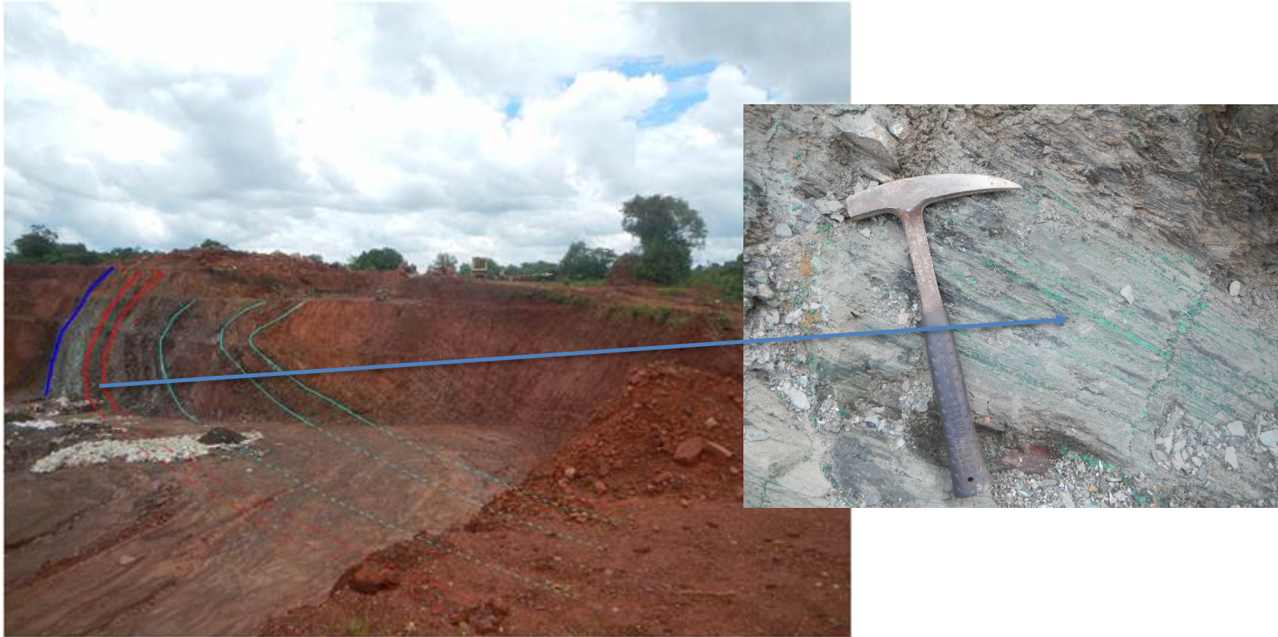
Kasombo 5 Prospect: image of pit showing bedding (with light blue line, downdip projection as dotted line); basal fault (dark blue line); mineralisation target (red lines, downdip projection as dotted line)
