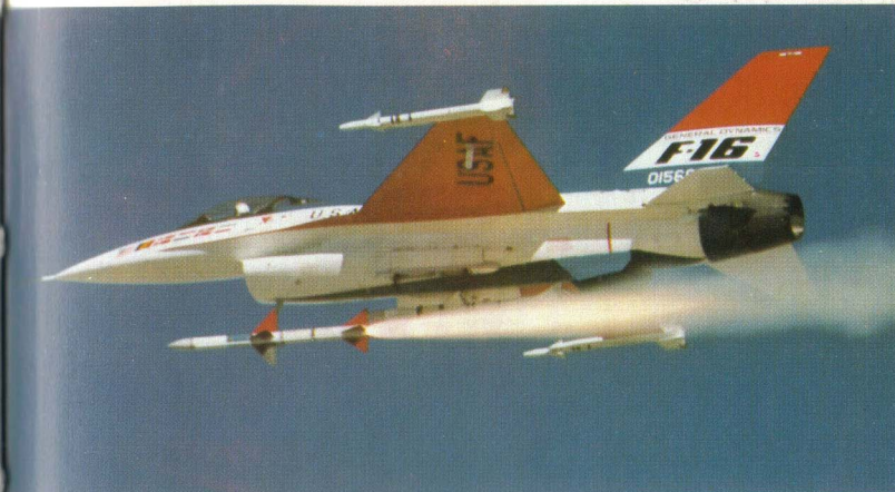
Above: Back in 1977 a prototype F-16 fired AIM-7F Sparrow missiles, which are not normally carried by these aircraft.
