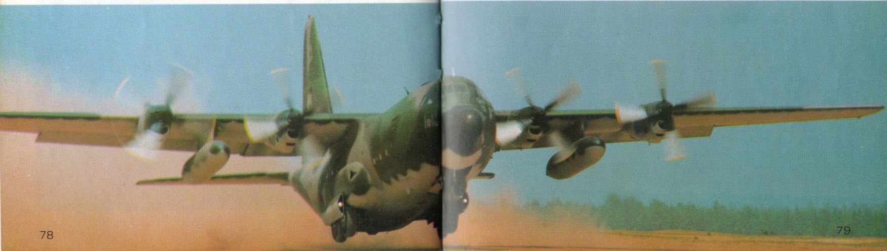
Below: All models of C-130 (this is a standard C-130H) are cleared for unrestricted weight operation from unpaved airstrips.
