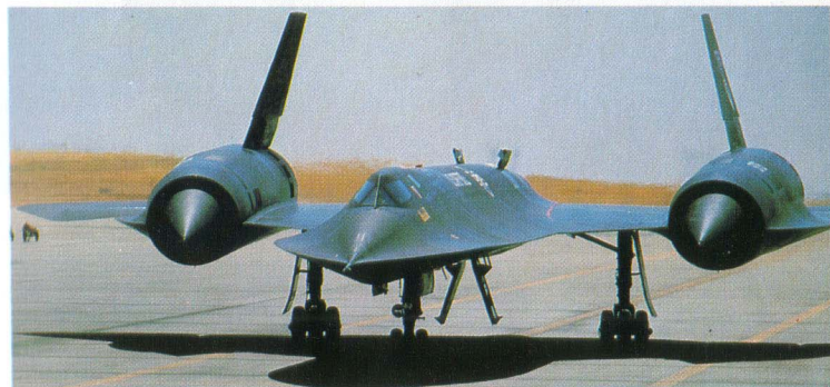
Above: A Blackbird of the 9th SRW taxis in at Beale after a mission, its braking-parachute doors still open above the body.
