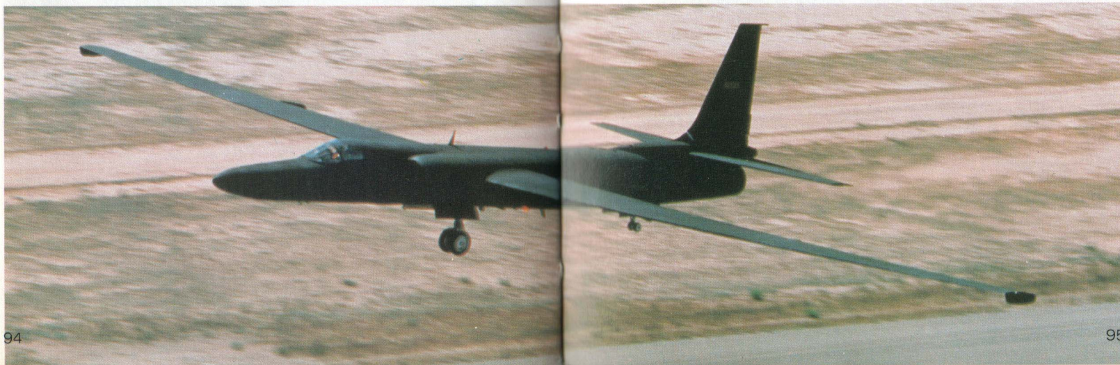
Above: Another of the many rebuilds was this black-painted example, believed to be a U-2L, originally the penultimate U-2B but converted for upper-atmosphere radiation measurements.
