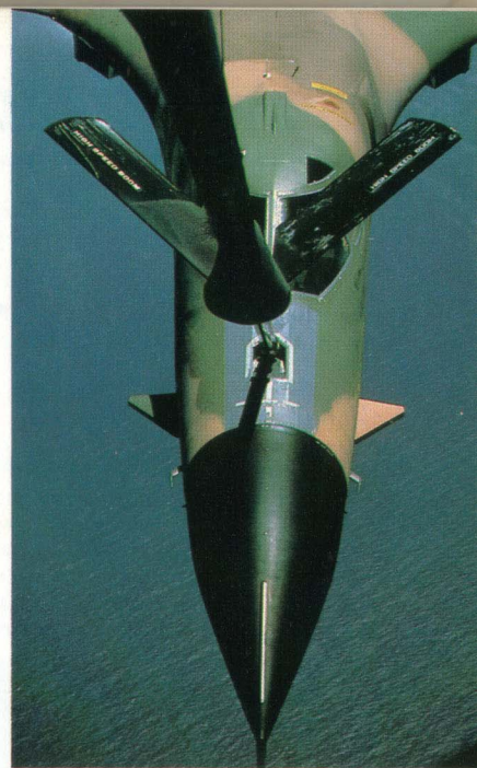
Above: Aerial refuelling, here of the third B-1A, extended the duration of test sorties.
