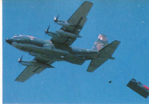
Above: Delivery from high level of an armoured car by parachuted pallet; the aircraft is a MAC C-130H.
