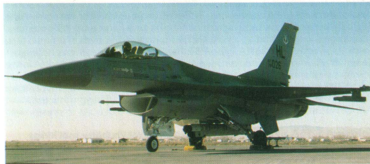
Above: Low-visibility F-16A with instrumentation transmitter on right wing and ALQ-119 jammer pod on centreline.
