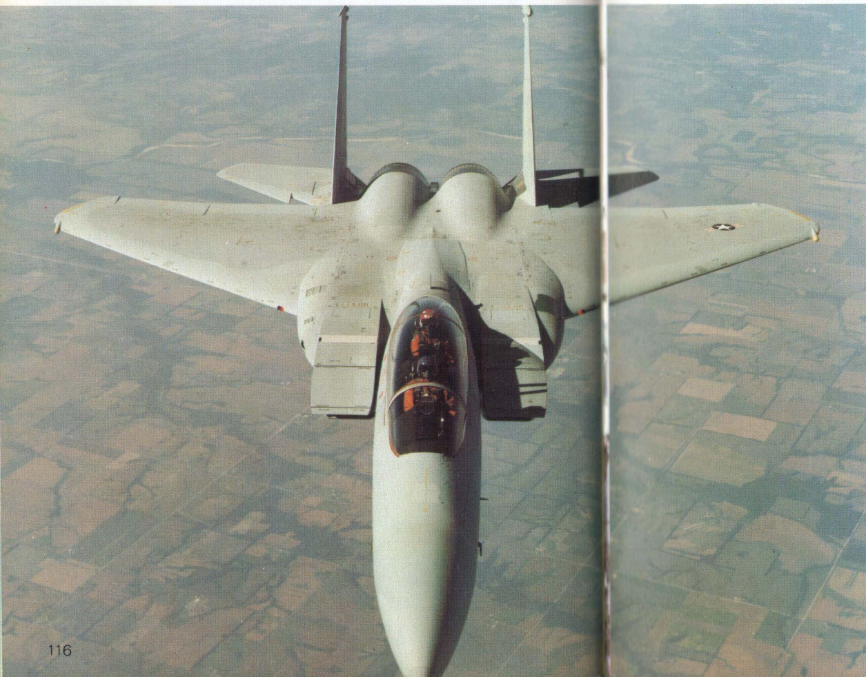
Left: F-15C in current low-visibility two-tone grey. The F-15 has large surface area in relation to its mass.
