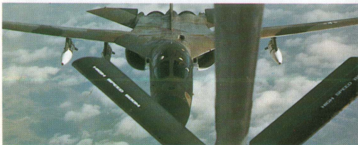
Above: Though called a Short-Range Attack Missile the AGM-69A (here carried by FB-111A) can fly ranges up to some 100 miles (160km).
