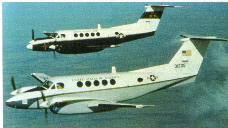
Above: A USAF VC-12A in company with a US Army C12-A Huron (rear). Both are variants of pressurized Super King Air.
