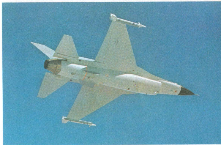
Above: In sharp contrast, this F-16A is flying in the minimum air-combat configuration, with no stores other than a pair of AIM-9J on the tip rails. Thrust/weight ratio can exceed unity.
