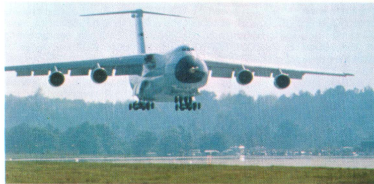
Above: Taken during manoeuvres with the USA in the United States this landing picture shows both the multi-segment flaps and the 28 landing wheels needed to confer 'flotation' for soft fields.
