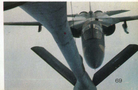
Below: View of an F-111 of TAC as it edges in under a KC-135 with its boom receptacle door open above the fuselage.
