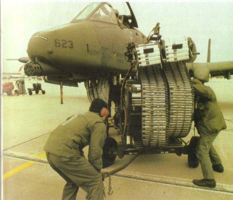
Above: By far the hardest-hitting gun in any air force is the GAU-8 of the A-10A; here ammo is loaded at the 354th TFW.
