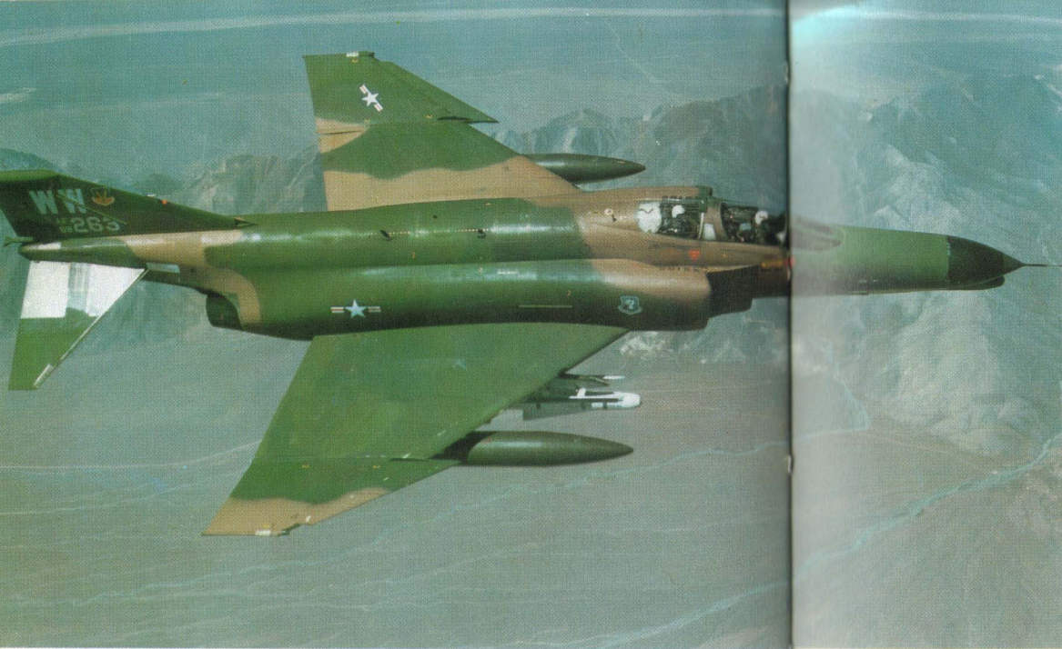
Above: This F-4E carries various advanced electronic systems for night ground attack, including the Pave Tack pod on the ventral centreline. The stabilised head of this pod contains a laser and FLIR (forward-looking infra-red) boresighted together and interfaced with the ARN-101 digital electronics on board the aircraft.
