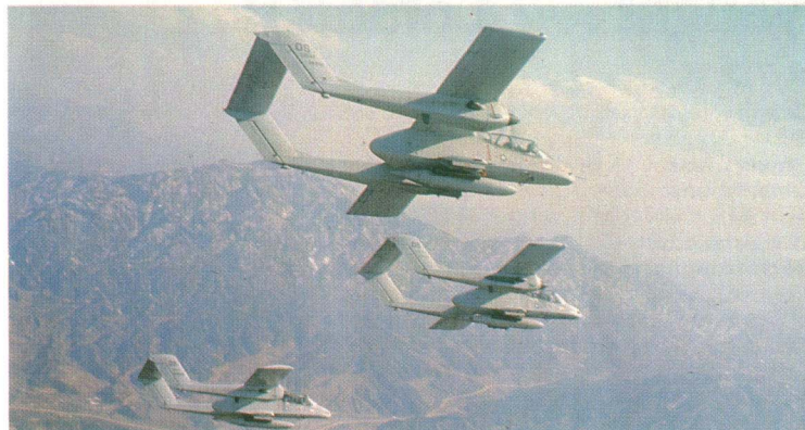
Above: The OV-10A has the capability of carrying almost all light tactical stores, these S. Korean-based examples having rocket pods.
