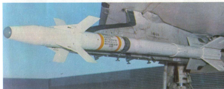
Above: Distinguished by its blunt double-delta control surfaces, the AIM-9J Sidewinder was replaced in production by the AIM-9L.
