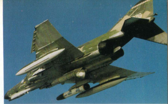
Above: This F-4E carries various advanced electronic systems for night ground attack, including the Pave Tack pod on the ventral centreline. The stabilised head of this pod contains a laser and FLIR (forward-looking infra-red) boresighted together and interfaced with the ARN-101 digital electronics on board the aircraft.
