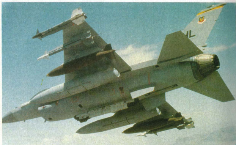
Above: An F-16A of the 388th burdened by two AIM-9L, two AIM-9J, two Mk 84 (2,000-lb, 907-kg) bombs, two 370-US gal (1700-litre) drop tanks and a Westinghouse AN/ALQ-119 (V) ECM pod.
