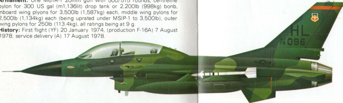
Left: An F-16B two-seater of the 388th TFW, Hill AFB. The AAMs are AIM-9J1 Sidewinders.
