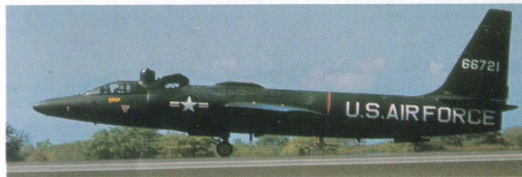
Above: Another of the many rebuilds was this black-painted example, believed to be a U-2L, originally the penultimate U-2B but converted for upper-atmosphere radiation measurements.
