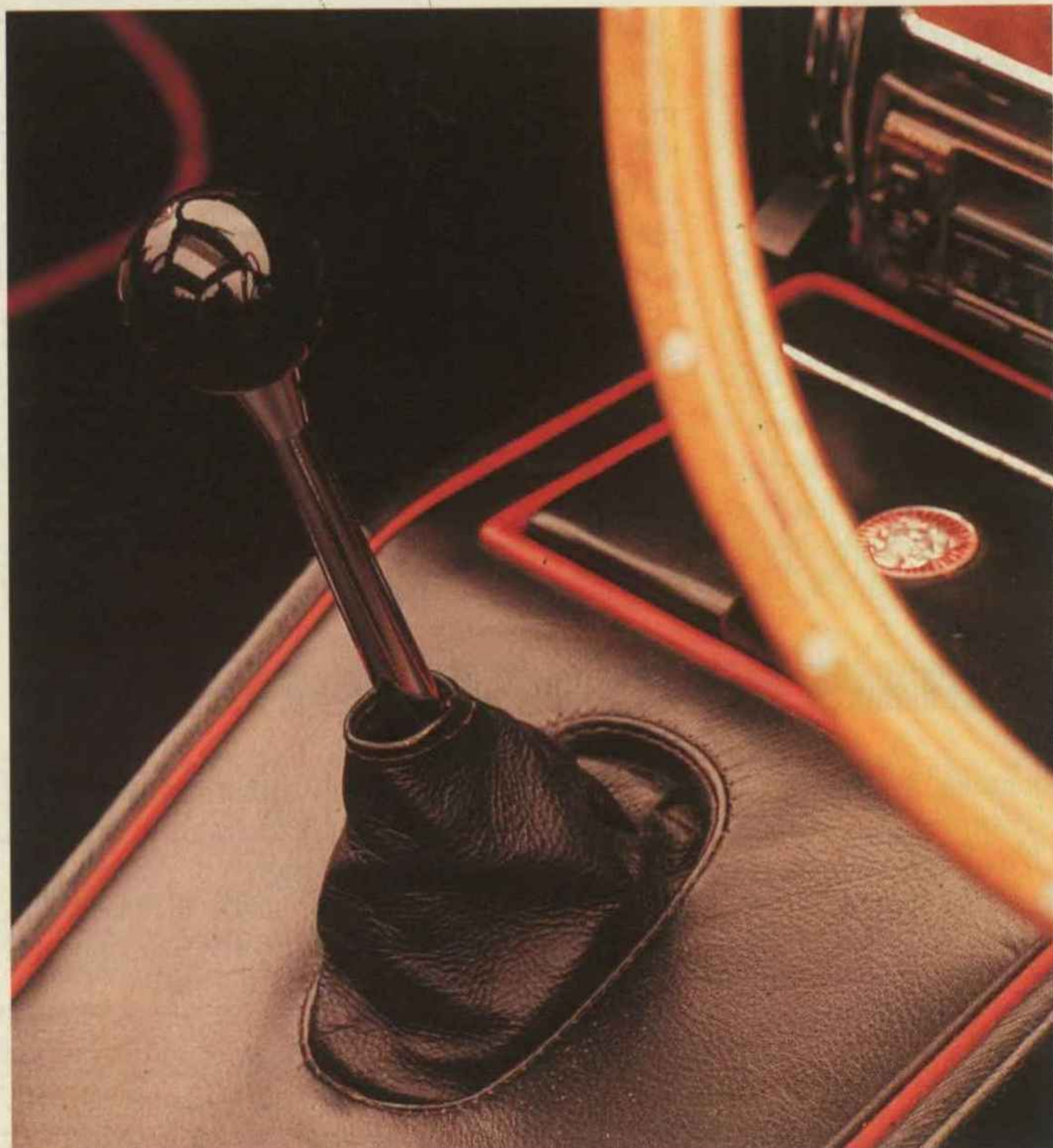
MkII gearbox in Coombs car is standard item; four speeds plus a column stalk operated overdrive. Ratios evenly spaced, great to swap between
