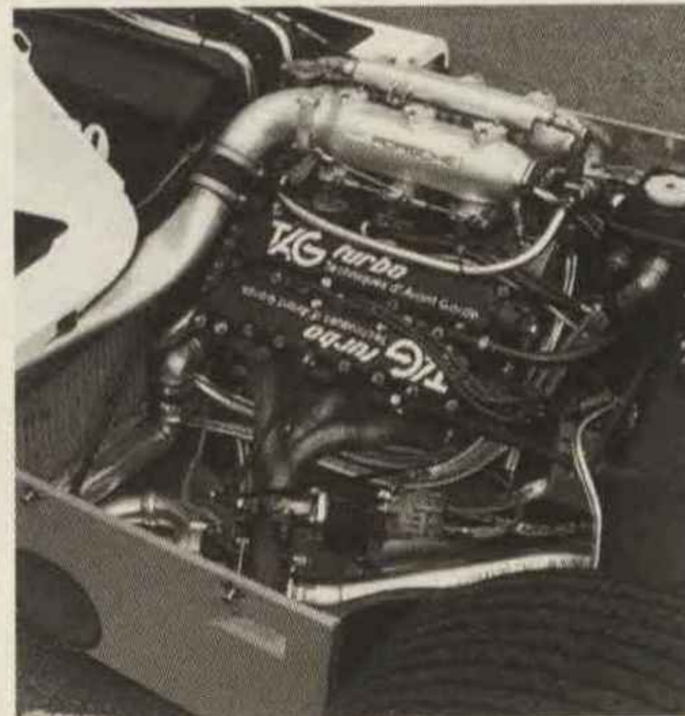
First Honda F1 mule has already been very fast in testing. Right: Porsche built McLaren's winning TAG turbos
