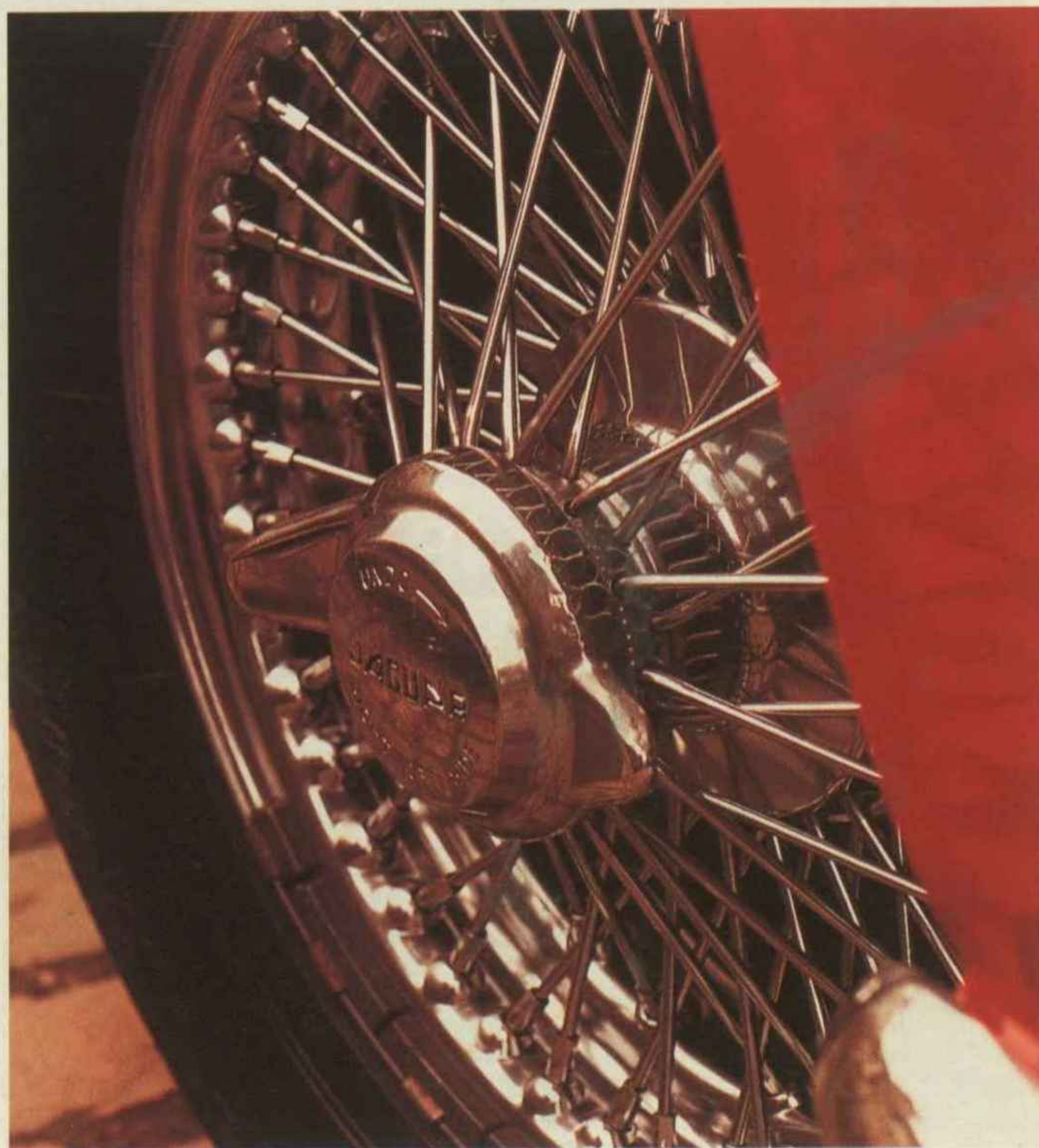
Beautiful spoked wheels come complete with centre lock knock-on spinners. Makes wheel changing easy, not great for unsprung weight
