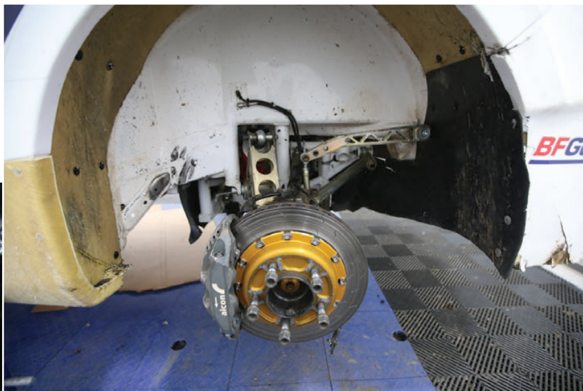
ABOVE & BELOW Unlike conventional rivals, the Civic uses inboard suspension with the damper mounted inside the chassis at a near horizontal angle (below right)
