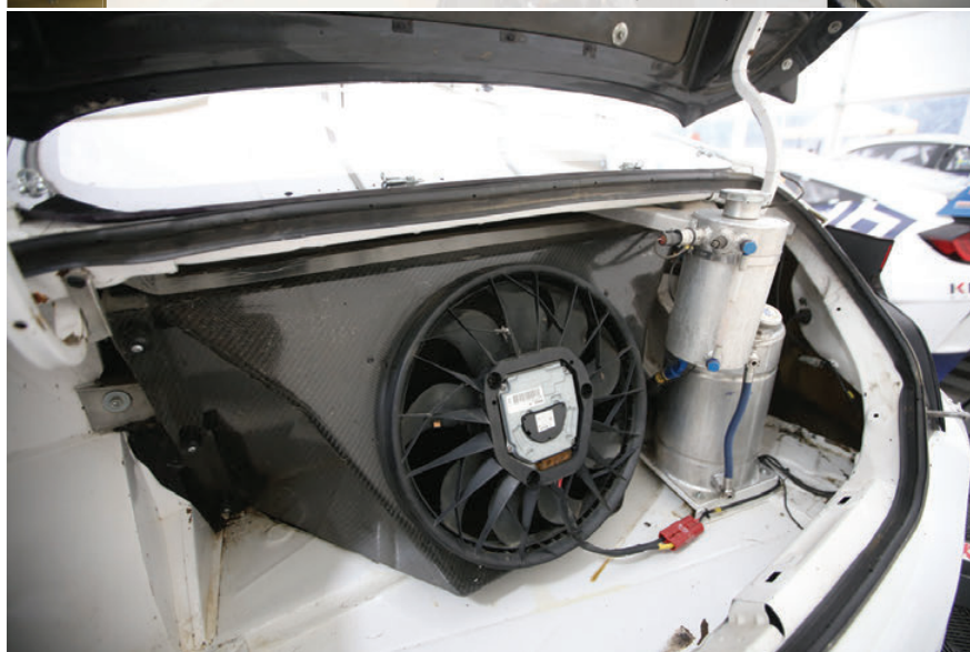
ABOVE & BELOW The radiator is relocated to the rear of the car, fed by ducts in the rear quarter panels, with warm air evacuated through the tailgate
