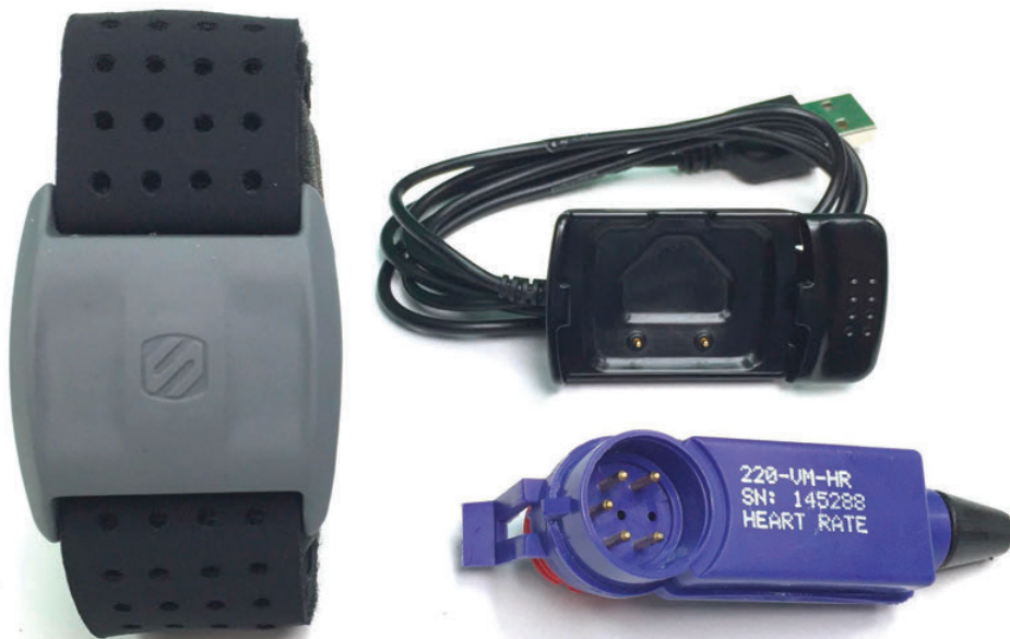
ABOVE Racepak's V-net heart rate sensor module hooks up to a data logger
