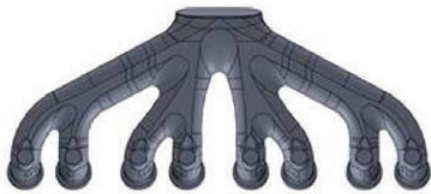
ABOVE Exhaust manifold showing unequal lengths of the primaries
