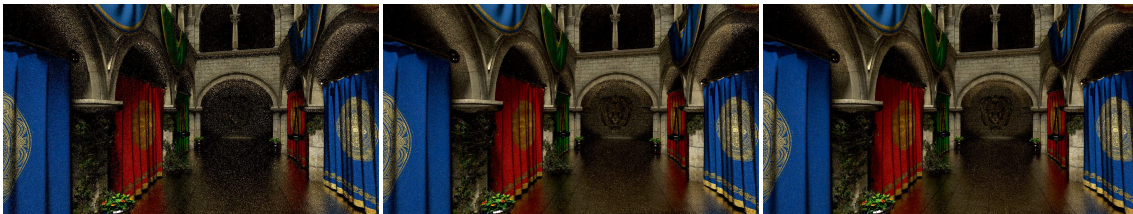
Figure 37: Comparison between the default path tracer (left 221ms), reprojection (center 201ms) and the combination (right 201ms).
