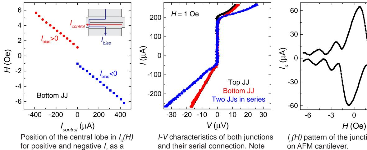
$I_{c}(H)$  pattern of the junction fabricated on AFM cantilever.
