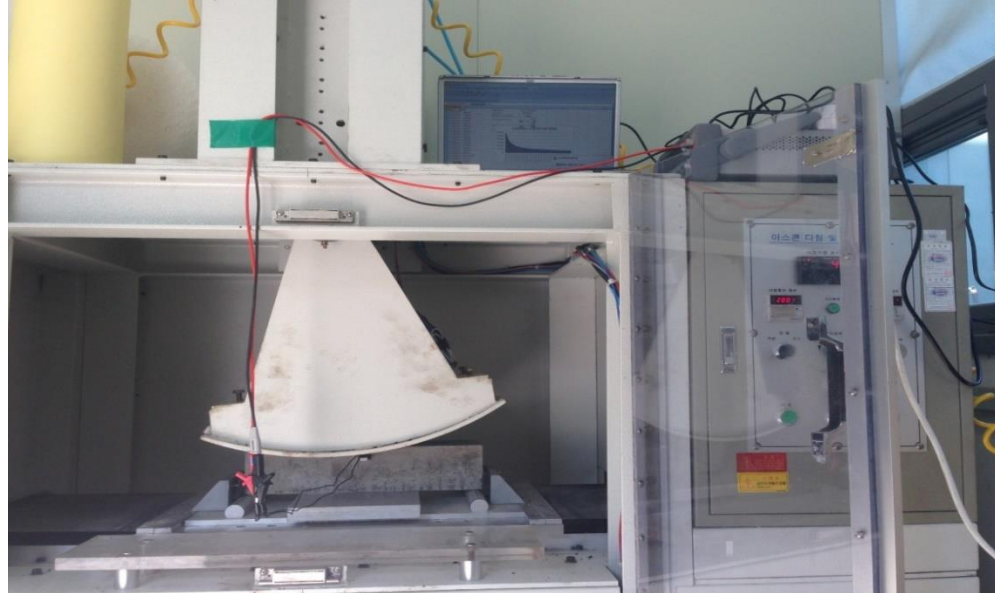
Wheel load test experimental set-up for 5 wt.% MWNT/PU composite (KCL institute)
