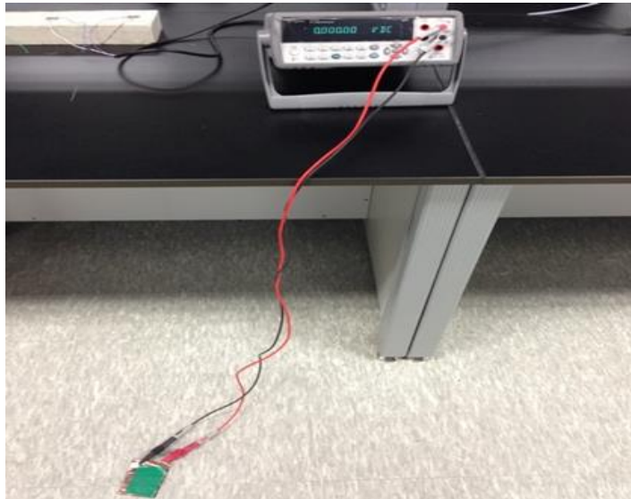
Experimental set-up of CNT/ZnO/PU voltage generator [15]
