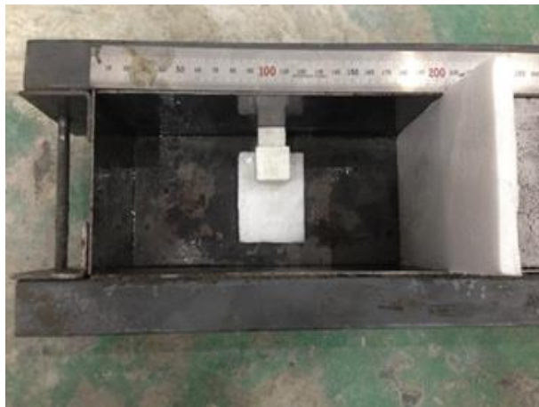
A mold used to fabricate piezoresistive sensors [13]
