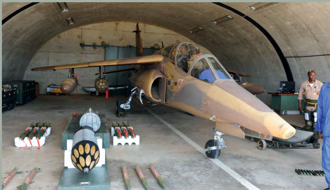
Above: An Alpha Jet in its hardened shelter at Garoua Air Base, with two of its main weapons on display: the Matra SNEB 68mm rocket launcher and BAP 100 bombs. All photos, Erwan de Cherisey unless stated Below: Personnel from the French company SOFEMA Aviation Services overhaul most of the CAF's aircraft at Garoua.
