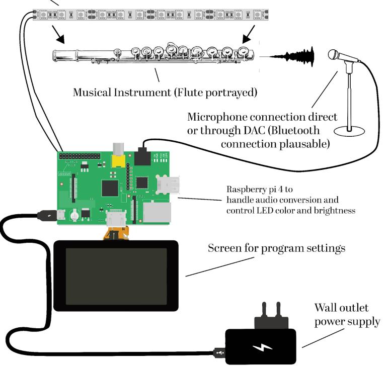
LED strip conected to, or imbeded inside instrument
