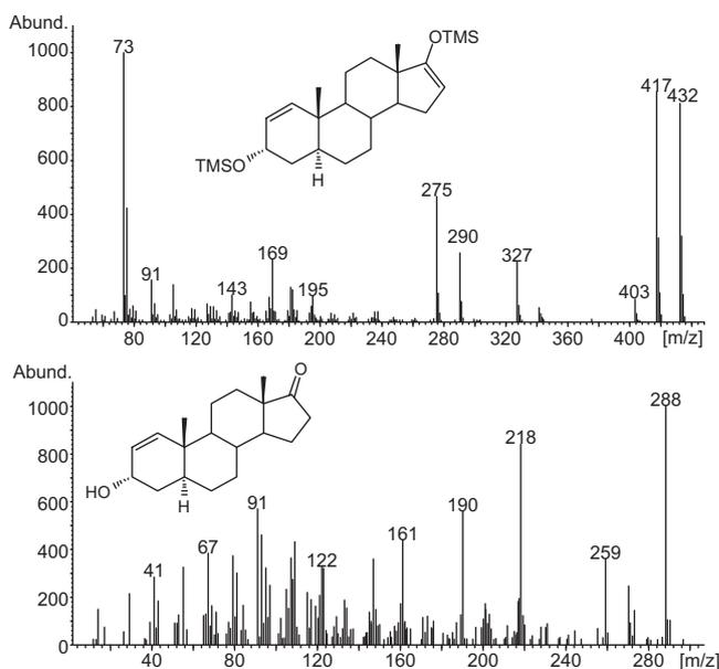
**Fig. 4.** Mass spectra of main metabolite, identified as 3 $\alpha$ -hydroxy-5 $\alpha$ -androst-1-en-17-one (**4**), upper bis-TMS,  $M^+ = 432$ , lower underivatized,  $M^+ = 288$ .
