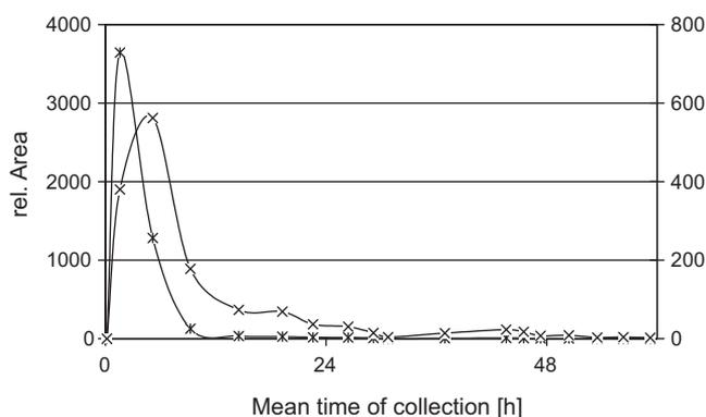
**Fig. 11.** Elimination kinetics of HO-Dione1 (\*, left y-axis) and HO-Dione2 (×, right y-axis) after one capsule of “1-Androsterone”, data shown using midpoints of collection periods and concentrations in 1000-fold peak area of analyte divided by area of internal standard.
