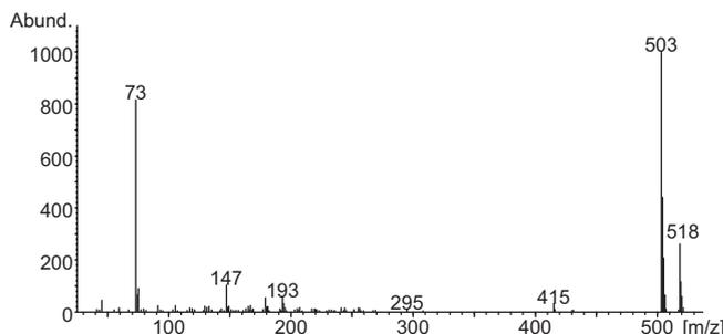
Fig. 7. Mass spectra of hydroxylated metabolites as tris-TMS derivatives upper: HO-Dione1 ( $M^+ = 518$ , RRT = 1.14), lower HO-Dione2 ( $M^+ = 518$ , RRT = 1.26).
