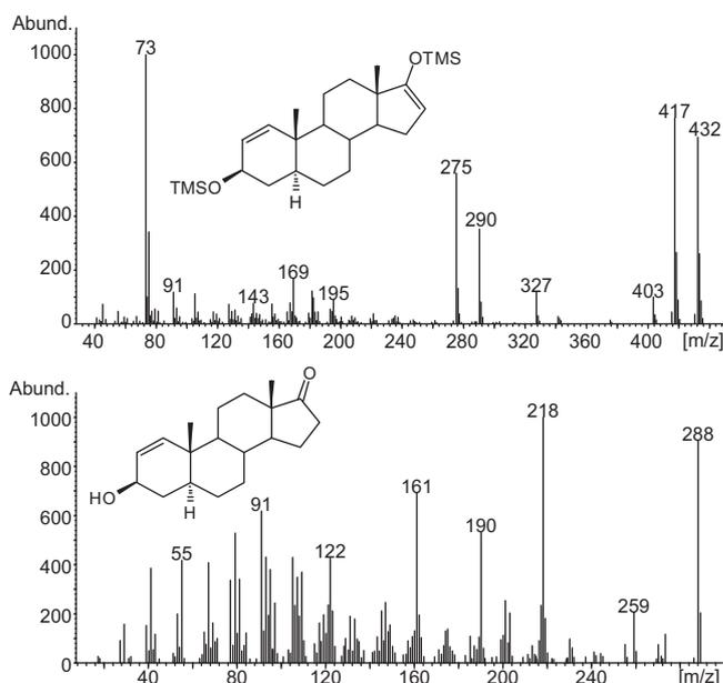
**Fig. 3.** Mass spectra of 3 $\beta$ -hydroxy-5 $\alpha$ -androst-1-en-17-one (**3**), upper bis-TMS,  $M^+ = 432$ , lower underivatized,  $M^+ = 288$ .
