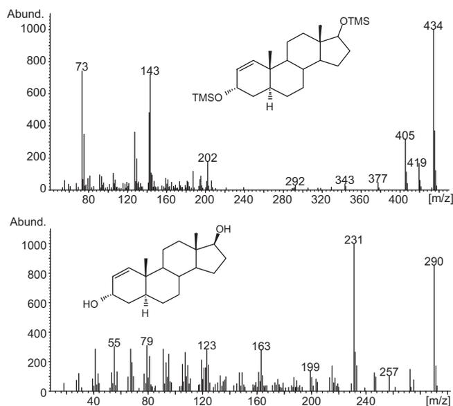
**Fig. 5.** Mass spectra of metabolite, identified as 5 $\alpha$ -androst-1-ene-3 $\alpha$ ,17 $\beta$ -diol (**5**), upper bis-TMS,  $M^+$  = 434, lower underivatized,  $M^+$  = 290.
