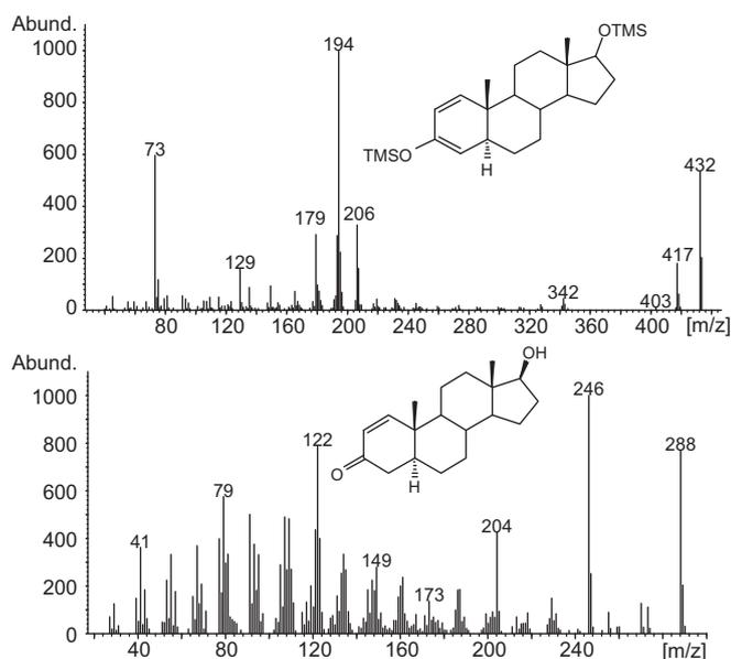
**Fig. 1.** Mass spectra of 17 $\beta$ -hydroxy-5 $\alpha$ -androst-1-en-3-one (1-testosterone, (**1**)), upper bis-TMS,  $M^+ = 432$ , lower underivatized,  $M^+ = 288$ .
