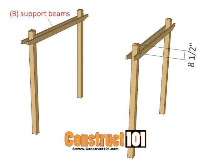
Install the support beams (B) as shown on illustration above, use clamps to hold the support beams in place, secure with 3 1/2" deck screws.
