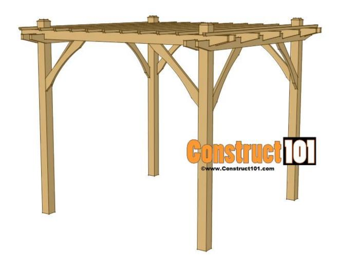
Install the brace (E) to the pergola using 3 1/2" deck screws as shown on illustration above.
