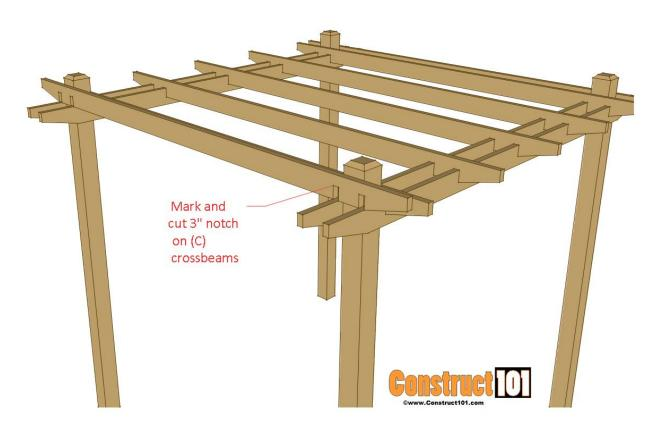
Lay the crossbeams (C) in place and mark were the 3" notch will go. Secure the crossbeams using 3 1/2" deck screws.
