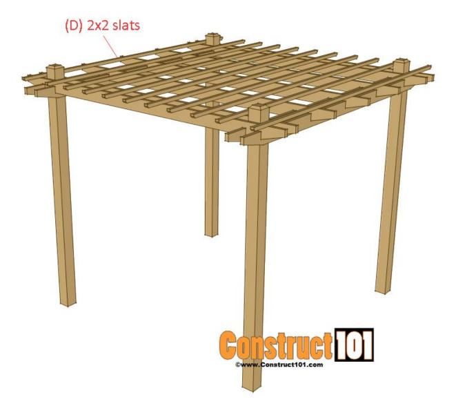
Use eleven 12' long 2×2's for the slats. The ends can be cut for a nicer appearance, illustration above shows end cut at 45 degree. Use 3 1/2" deck screws to secure the slats.
