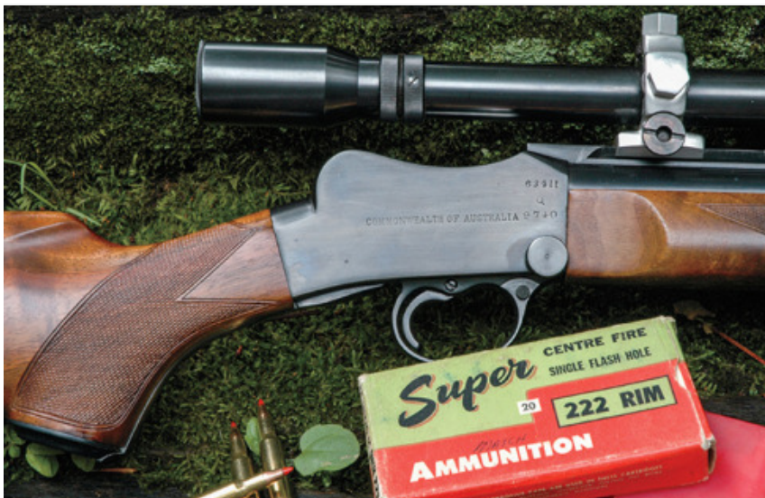
Simpson's custom single-shot rifle on a Martini Cadet action is chambered for a rimmed version of the .222 Rem. often referred to as the .222 Super.
