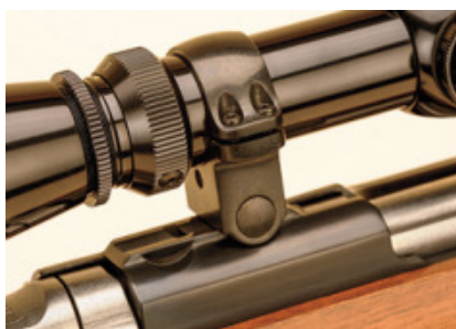
There are two locations behind the ejection port to attach one of Ruger's supplied proprietary rings, which provides plenty of latitude for scope mounting.
