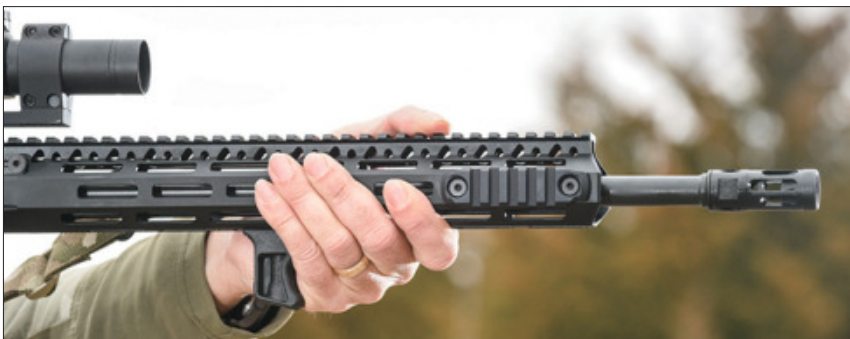
The chrome-lined barrel is fluted and sports a 1:7 twist. The handguard is a Bravo Company 13-inch MCMR free-floating model.
