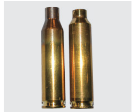
The .26 Macho's parent case is the .260 Rem. (l.), with a 30-degree shoulder that was pushed forward about .080 inch.
