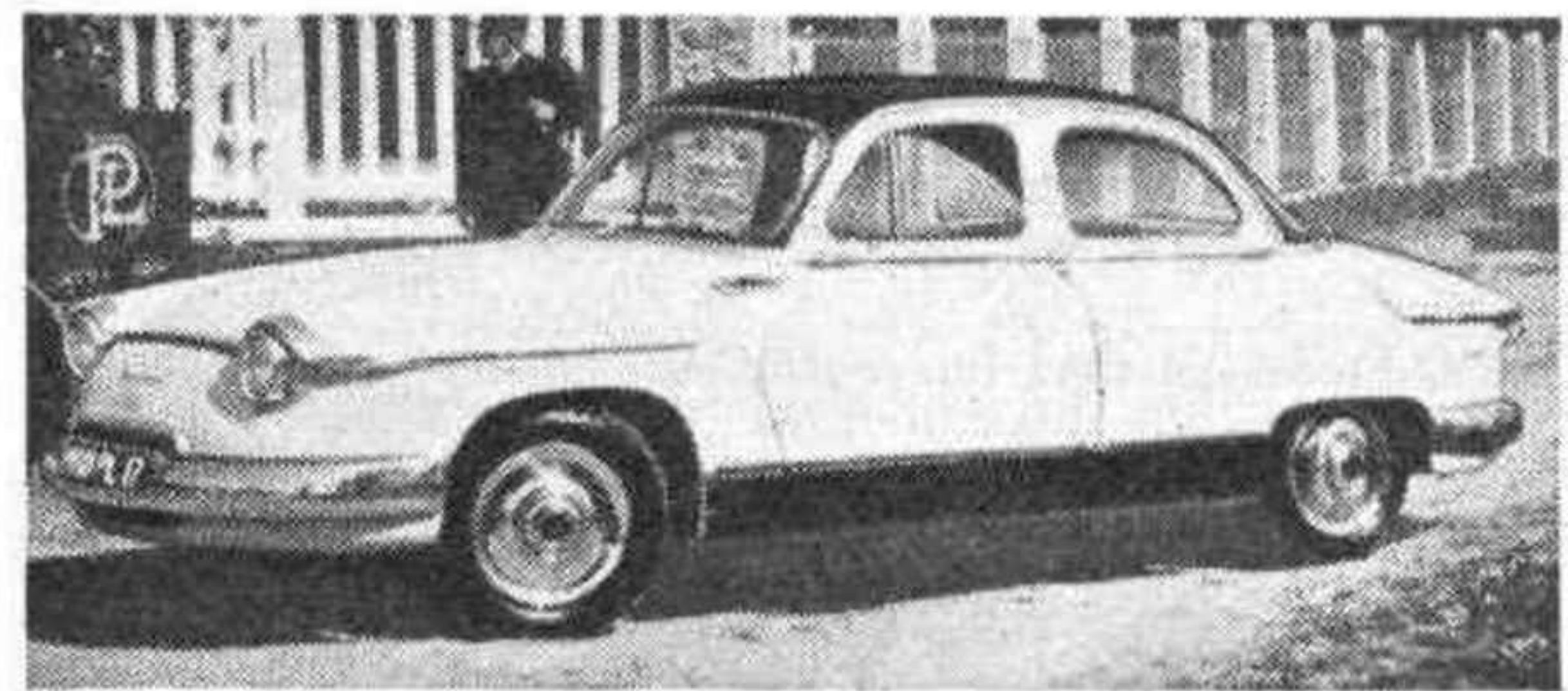
ANOTHER 850 c.c. f.w.d. small car, the Dyna-Panhard is seen here in its latest PL.17 form.
