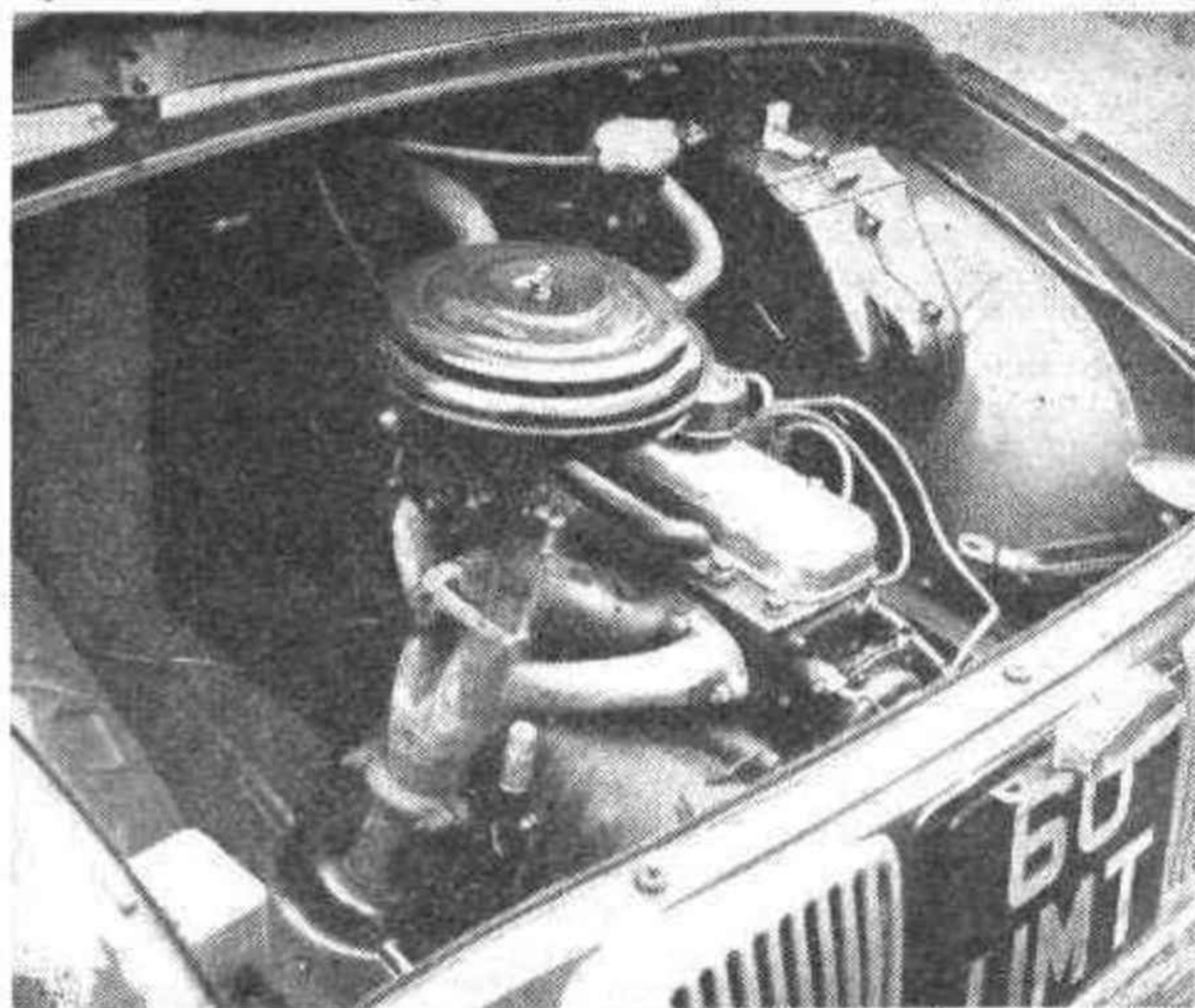
THE ENGINE of the Dauphine Gordini, showing the revised manifold and polished valve cover, etc. It gives 8 b.h.p. more than the normal version.
