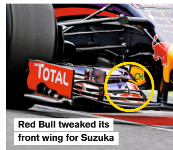
Multiple elements help reduce airflow separation
