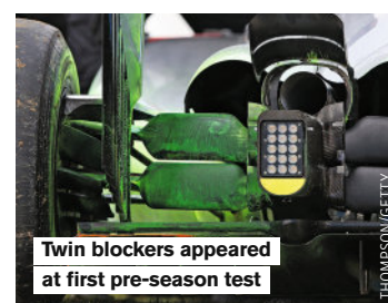
Lower suspension blocker worked OK on the McLaren
