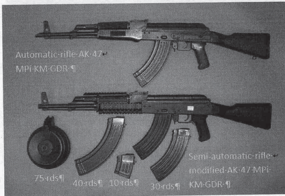
Pic. 5: Semi-automatic rifle MPI-KM, modified from full-automatic rifle AK-47/MPI-KM, former GDR, cal. 7.62mm x 39 ¶
