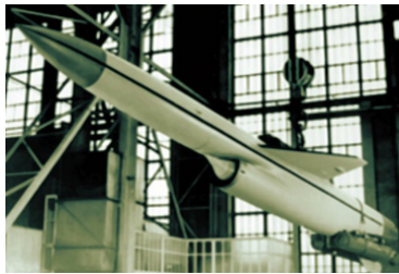
Figure 1.28. The P-500 (4K80) Bazalt missile (source: rights reserved)
