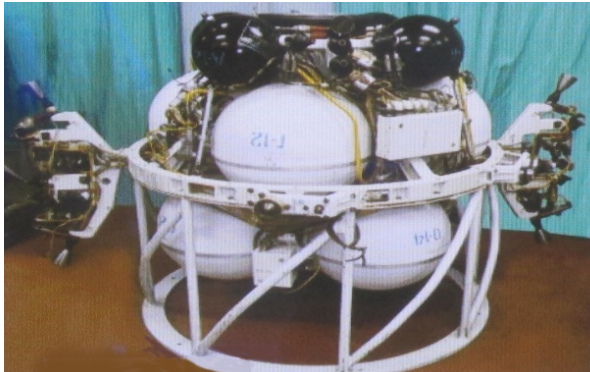
Figure 2.33. The 4E18 engine from the US satellite (source: rights reserved). For a color version of this figure, see www.iste.co.uk/lardier/proton.zip
