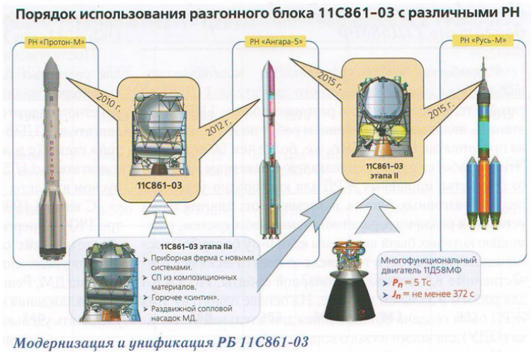
Figure 4.19. Steps 1 and 2 of the Bloc-DM-03 stage (source: all rights reserved). For a color version of this figure, see www.iste.co.uk/lardier/proton.zip
