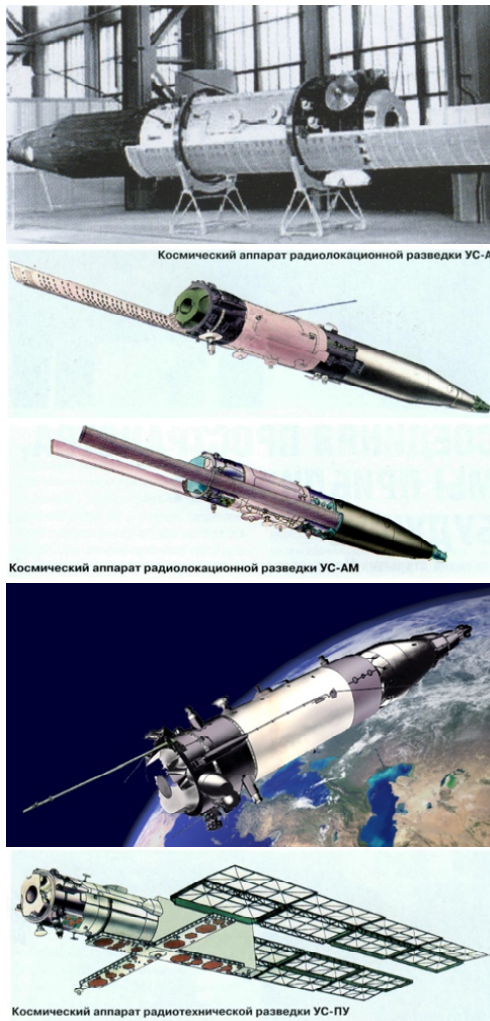
Figure 3.17. The US, US-A, US-AM, Plasma-A and US-PU (source: NPO Mash, KB Arsenal). For a color version of this figure, see www.iste.co.uk/lardier/proton.zip
