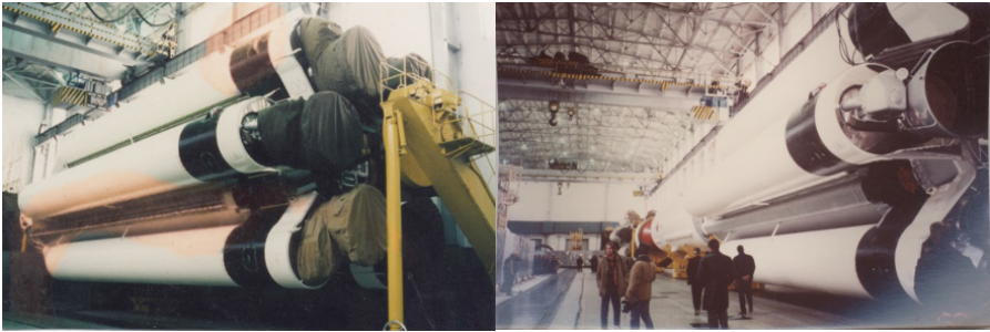
Figure 4.12. Proton assembly in the MIK (source: Christian Lardier)
