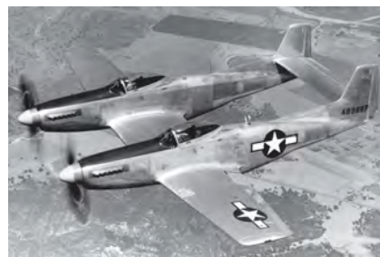
XP-82 44-83887 was the second Twin Mustang prototype. Both XP-82s and early production P-82Bs were powered by V-1650s before the Allison V-1710-100 was substituted. USAF
