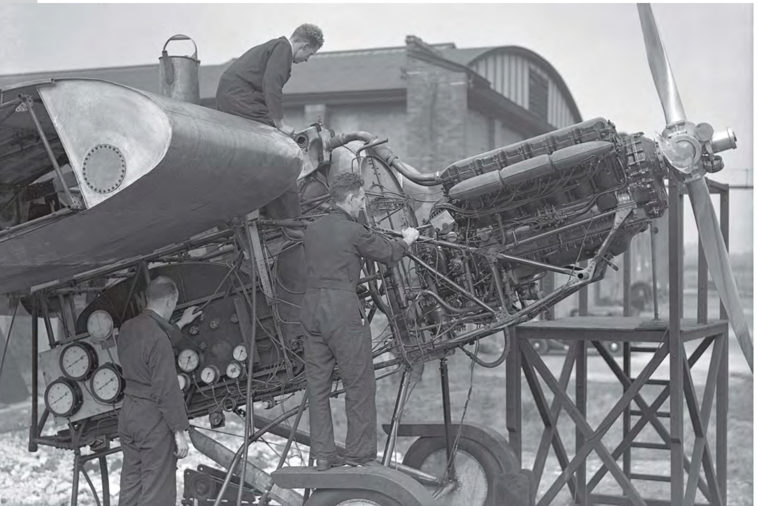
An instrumented external Merlin test rig at Rolls-Royce's Hucknall, Nottinghamshire-based experimental department. AEROPLANE
