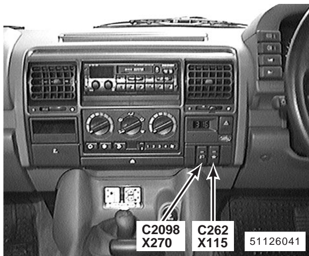
116. centre of fascia X115 Cruise Control Switch X270 Front Fog Lamps Switch C262 (5-U) C2098 (5-G)
