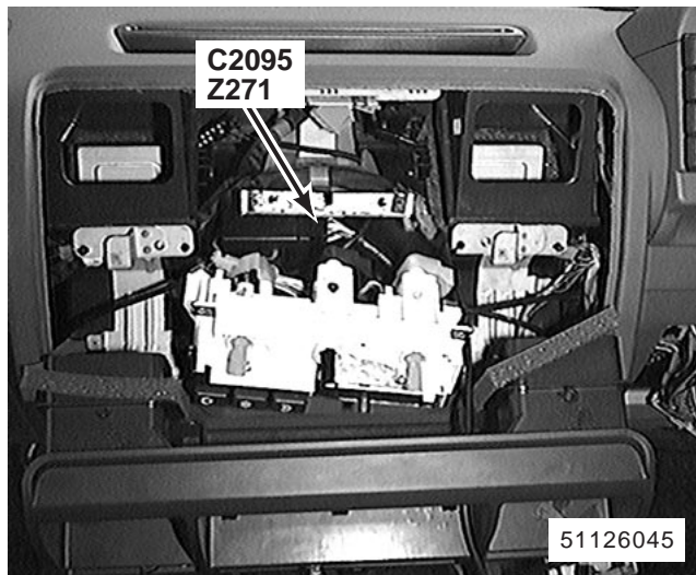
119. behind centre of fascia
