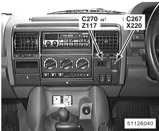
115. centre of fascia X220 Hazard Switch Z117 Clock C267 (10-W) C270 (4-B)
