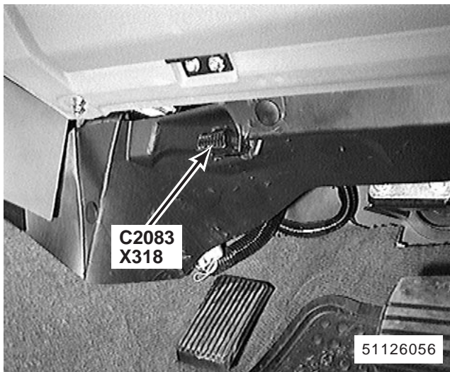
135. behind RH side of fascia left of steering column X318 Data Link Connector (OBDII) C2083 (16-S)
