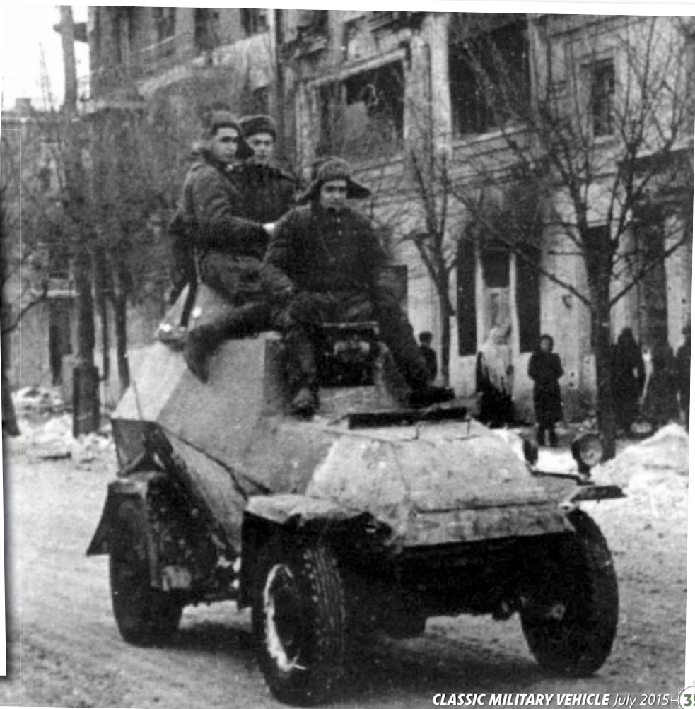
Right: A BA-64 with its narrow track photographed in February 1944. Below: A May 1942 photo of an early BA-64. There are no driver's side vision ports.
