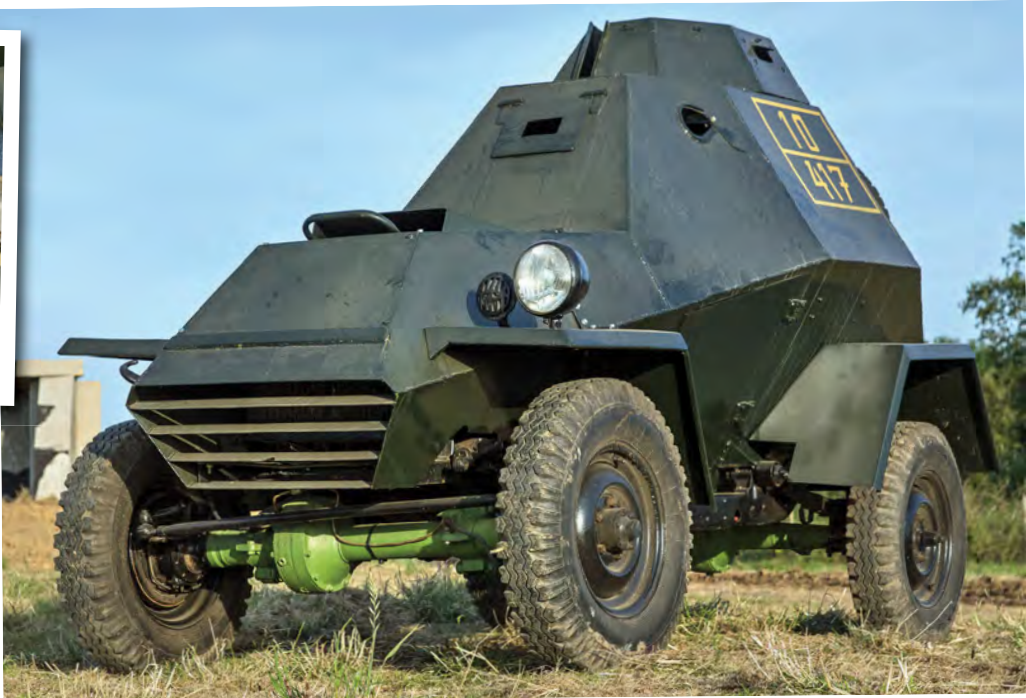
Right: With armour plate up to 15mm thick, the BA-64 was noticeably top heavy, so Nick and James used 3mm mild steel when they fabricated the new body. With only a small vision flap to his front and small vision ports either side, the driver's view is limited.
