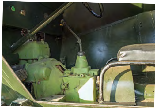
Above: The BA-64's driver sat centrally, astride the transmission.
