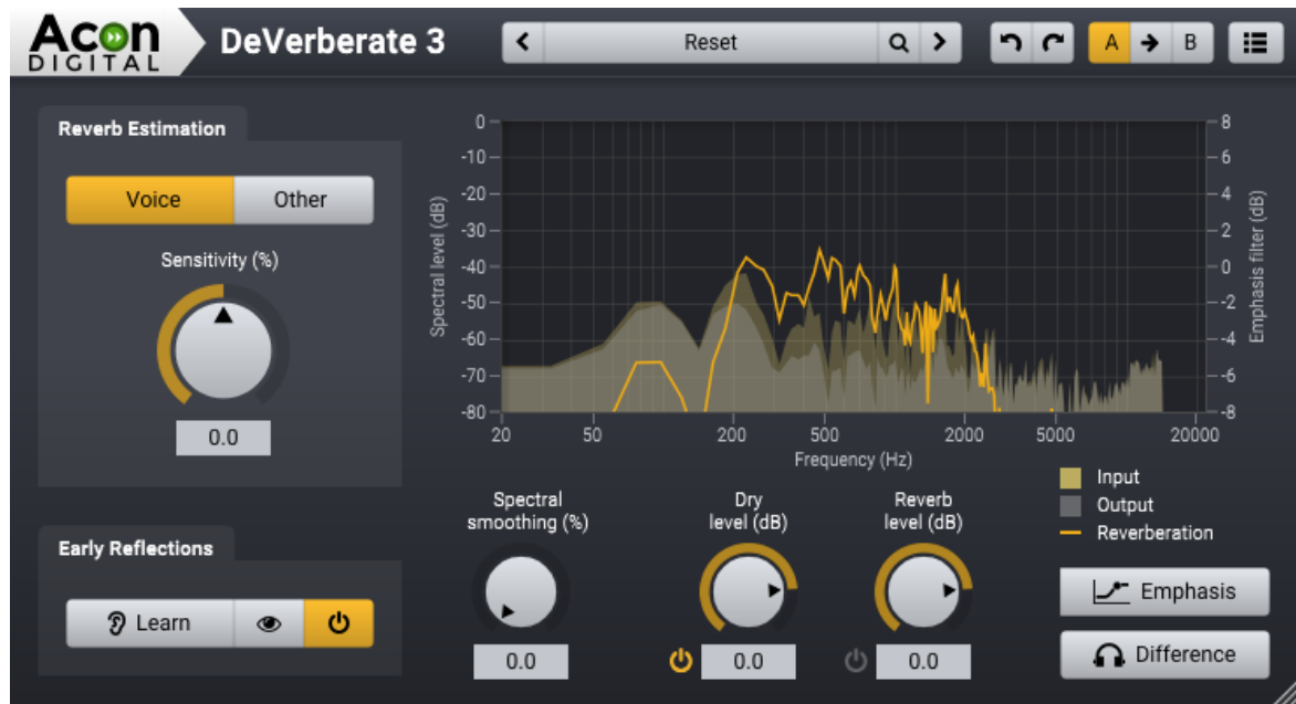
The DeVerberate plug-in running in Voice mode. The graph shows the estimated spectrum of the reverb as well as the frequency spectrum of the input and output signals.
